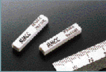
Wide-band, high-gain chip antennas
