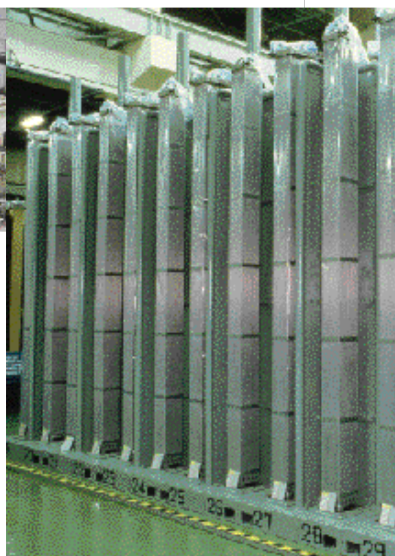
Nuclear fuel assemblies fabricated by Mitsubishi Nuclear Fuel Co., Ltd
