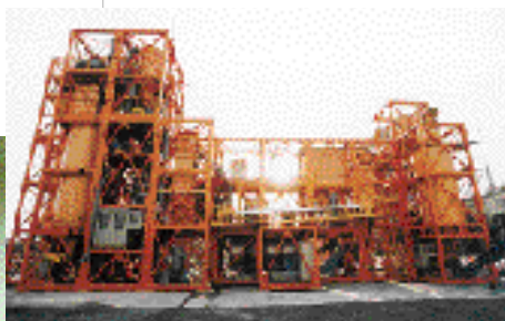
Moveable system for recovering high-quality aggregate
