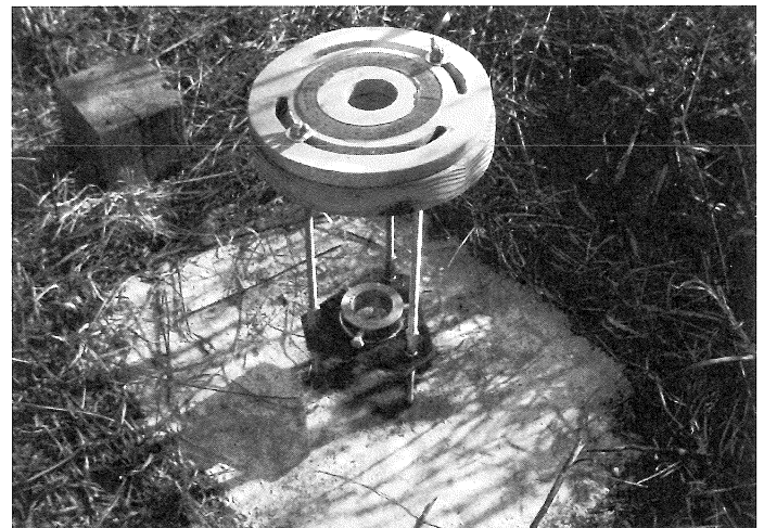
Figure 2. Compass rosette and steel thrust bearing connected to concrete base via 0.9525 cm all-thread rod.
