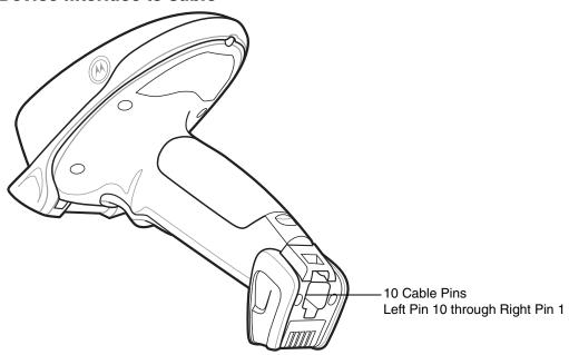
Figure A-2 Digital Connection Pins
