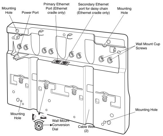
Figure 2-13 Four Slot Cradle - Back View
