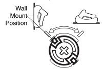
Figure 2-14 Wall Mount Conversion Dial - Wall Mount Position
