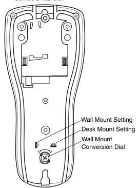
Figure 2-4 Set Conversion Dial for Wall Mounting
