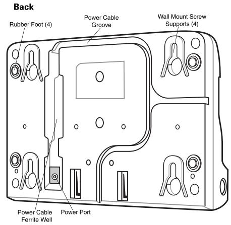
Figure 2-20 Four Slot Battery Charger - Back
