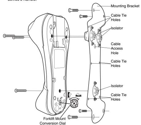
Figure 2-10 Attaching Forklift Mounting Bracket to Cradle
