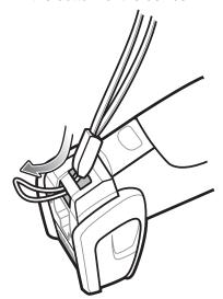
**3.** Pull the clip through the loop over the tether point and tighten into place.
