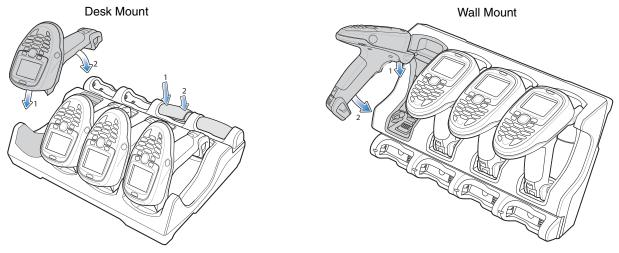
Figure 2-18 Inserting Devices
