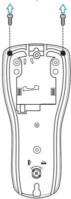
Figure 2-5 Remove Back Screws
