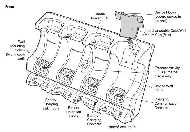
Figure 2-12 Four Slot Cradle - Front View
