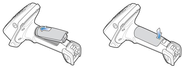
Figure 1-3 Battery Insertion
