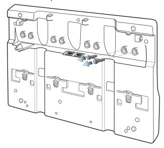
Figure 2-15 Remove Screws
