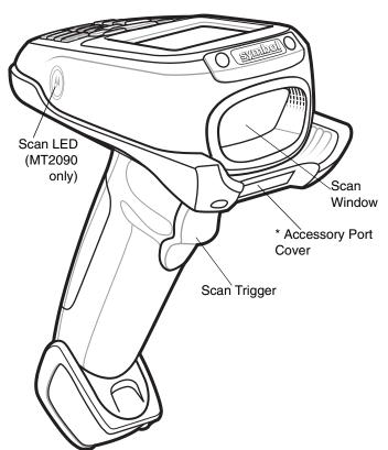
\* **Note:** The accessory port is not available for use at this time. The device is not water sealed if the accessory port cover is removed.
