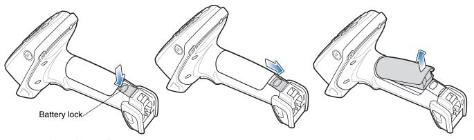
Figure 1-5 Li-ion Battery Removal
