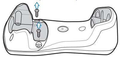
Figure 2-7 Remove Front Screws
