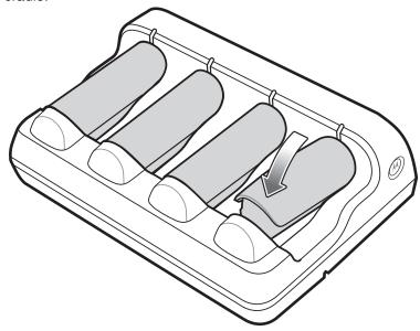
Figure 2-21 Inserting Batteries
