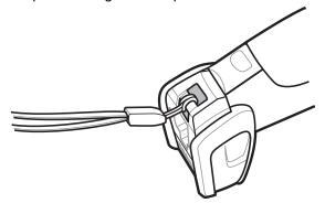
Figure 1-6 Attaching the Lanyard
