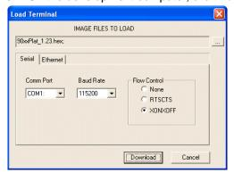
Figure 6-9 Load Terminal Window - Serial Tab
