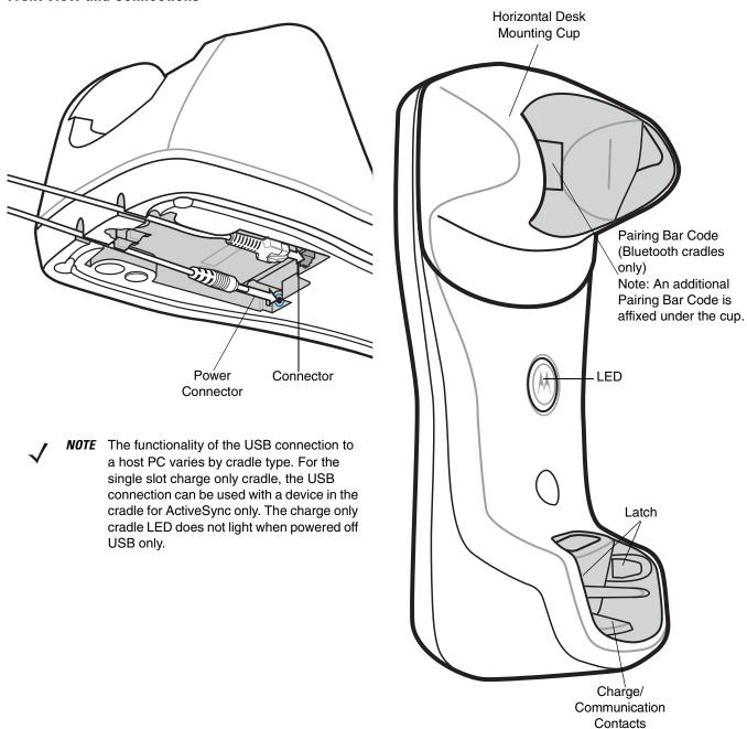
Figure 2-1 Single Slot Cradle - Connections/Pairing Bar Code
