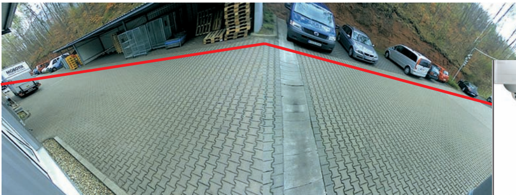
D12D-180° tilted too far down: Level area seems to buckle
