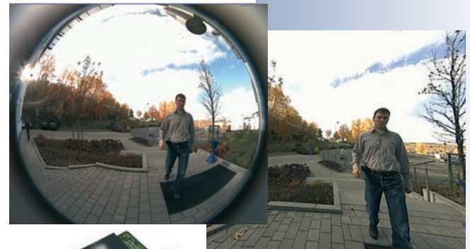
Image section with correction of wide-angle distortion
