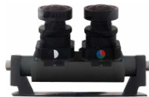
2 lens units on lens bridge Day&Night
