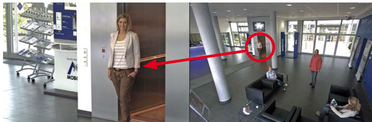
Original image: tele lens (left) and wide-angle lens (right) – simultaneously in one image
