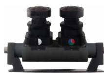
2 lens units on lens bridge Day&Night
