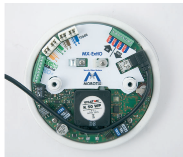
Insert USB plug Properly guide the cable
