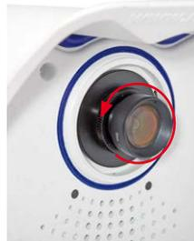
3. **Screw the new lens** (if present) back into the camera and restore the **power supply** of the camera.
