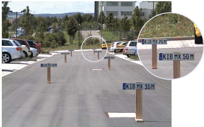
The image area captured by the camera varies depending on the selected lens (see *Section 1.3, «Technical Specifications»*). With a **Super Wide Angle lens** (e.g., L25 with 82°), for example, almost an entire room can be recorded from one corner. An **L160 Tele lens** enables an M25M with a high-resolution 5 megapixel sensor to clearly record a license plate number, for example, from a distance of approximately 75 meters.
