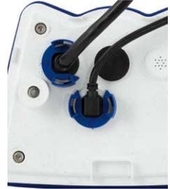
**Removing the Cable Retainer**
