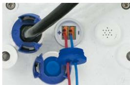
If you need to remove one of the wires, unlock the connector by pressing on the orange-colored area using a small screwdriver, then pull out the wire.
