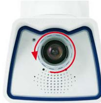
2. Remove the **lens** by turning it counter-clockwise.
