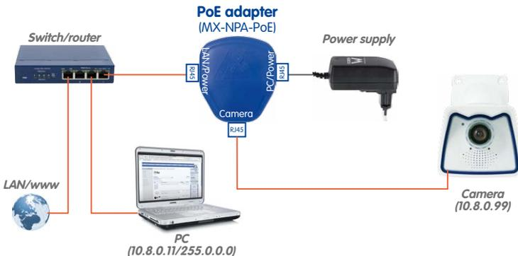
For the M25M you should use the blue MX-NPA-PoE-Set or the MX-NPA-Box - previous MOBOTIX network power accessories, such as the NPA-Set, Power-Box and Power-Rack (MX-NPA-Set, MX-NPR-4 and MX-NPR8/20) are not suitable for use with the M25M
