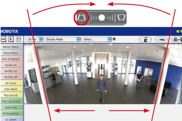
Depending on the mounting position (ceiling, wall, floor), panorama correction and mounting error correction may not be available!
