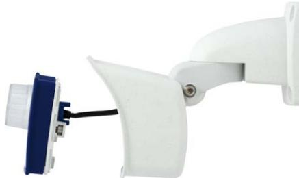
Depending on the later tilt of the camera, drill through the front or rear drain hole of the camera's weatherproof housing.
