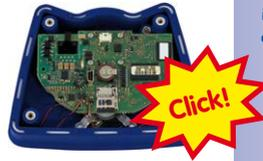
2. **Mount the back plate:** Replace the back plate of the camera housing, ensuring that the back plate screw holes are correctly positioned above the thread inserts.
