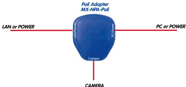
When directly connecting to the computer, the PoE adapter replaces a cross-over cable
