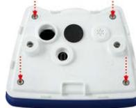
3. **Screw the back plate tight and replace the connection cables:** Place the four Allen screws back into the back plate and tighten the screws using the supplied 2.5 mm Allen wrench. The previously removed cables must now be reconnected (see *Section 2.7.5* and *Section 2.7.6*).
