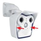
Using the supplied 5 mm Allen wrench, tighten the two bolts at the back of the camera housing. Push the two rubber plugs back into the opening of the screws to prevent humidity and dirt from entering the camera.
