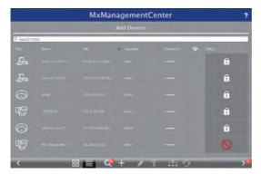
MxManagementCenter automatically monitors and displays the operating status of all cameras. Cameras that are not on the same subnet as the computer are indicated by the Licon (Camera not in the same network as the computer). Likewise, the cameras that have an unknown password or for which no user name/password combination has been specified in MxManagementCenter will be displayed with the icon (Camera is password-protected).
