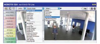
Camera live image withoutMOBOTIX panorama correction with Ouick Controls visible
