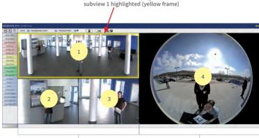
Left camera image with three subviews Panorama/Focus display mode (for example, Cam1 sensor module)
