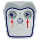
Connect sensor module cable: Firmly push the sensor module cable into the module's connector as shown in the figure.
