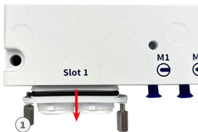
Fig. 23: Remove cover from interface board slot
