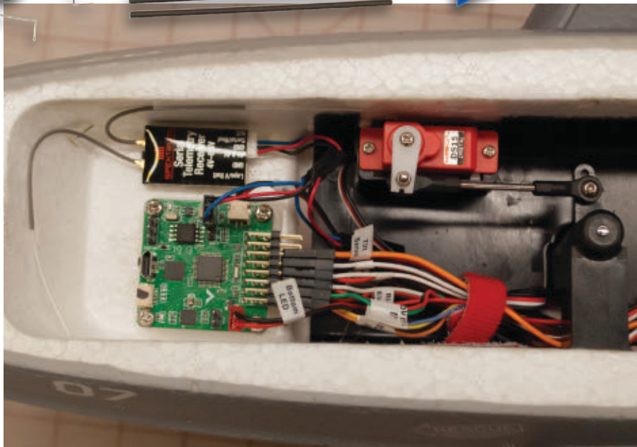
This flight controller (green circuit board) is the key to the FV-31's broad flight capabilities.
