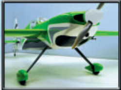
Painted fiberglass cowl & wheel pants with carbon fiber landing gear
