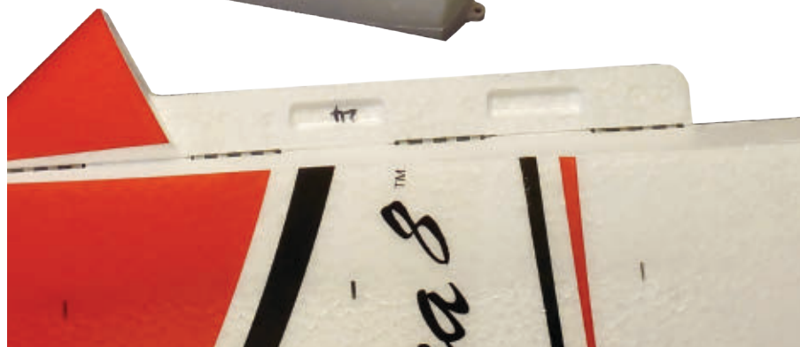
The rudder "snaps" together and is permanently attached with epoxy.
