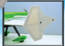
Removable Side Force Generators add stability to Knife-Edge & 3D flight
