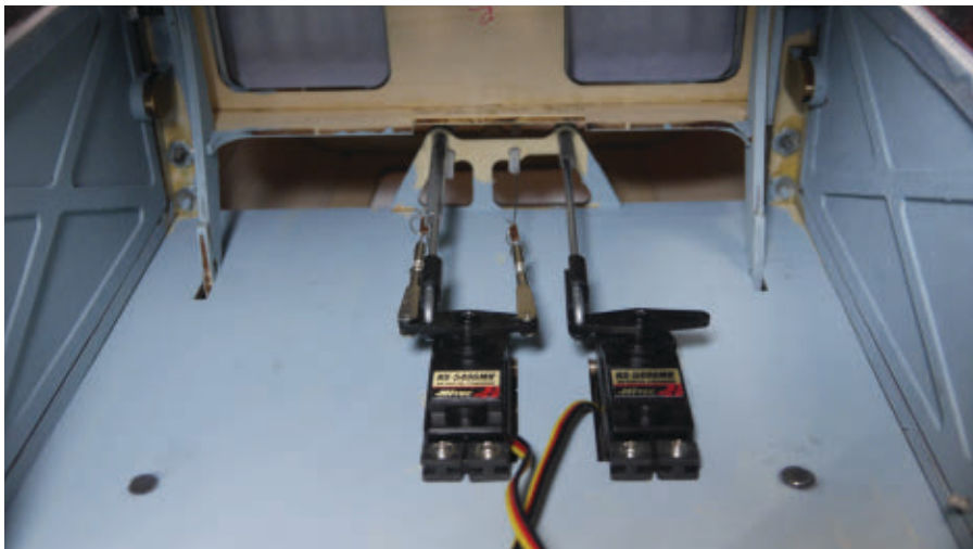
The Hitec elevator and rudder servos are cleverly hidden under removable seats.
