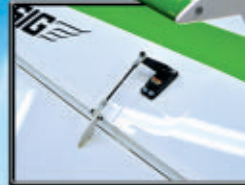
Surface mounted ailerons servos & ball links make installation easy
