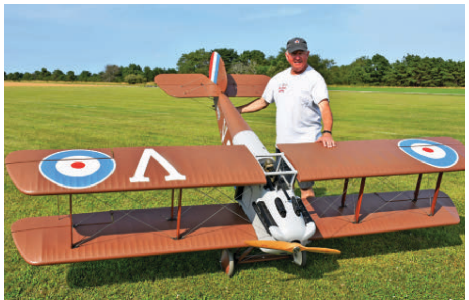
Roy Vaillancourt is shown with his 1/3-scale Sopwith Dolphin. Check out the reverse wing stagger.
