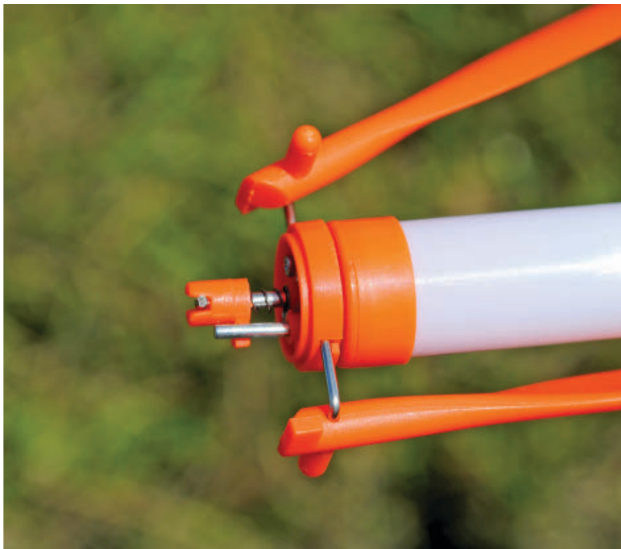
Removing the spinner reveals the workings of the reverse Montreal front end, which acts as a waiting stop with the motor wound and as a propeller stop at the end of the run to ensure that the blades fold under the wing.
