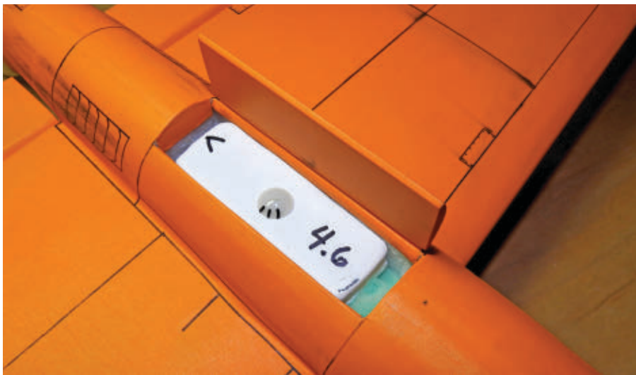
Full ballast is installed on the SR-48 using a 10-24 nylon bolt. The ballast is fully internal and located on the CG with the hatch.
