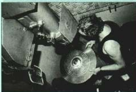
This overhead view illustrates how cymbals are hand-guided by the operator on the hammering machine.
