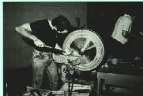
A lathe operator carefully shaves minute amounts of metal off a cymbal until the proper thickness is achieved.
