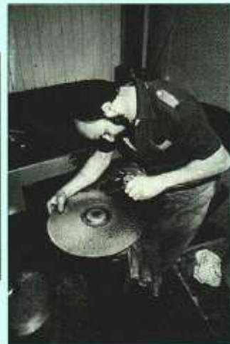
Following machine hammering, every cymbal gets "fine-tuned" by hand.
