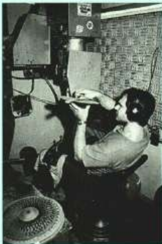
Each cymbal is frequently checked during the hammering process to ensure the proper profile.
