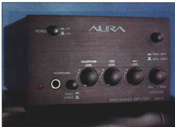
The AMP-75 is a compact yet sophisticated mixer that permits versatile self-monitoring control.
