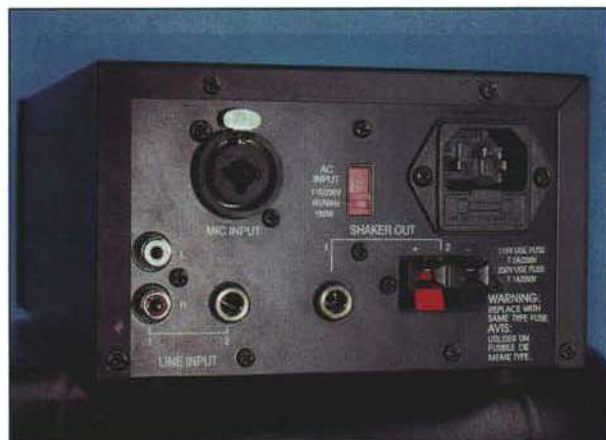
The back panel of the AMP-75 . The single mic' input can accept either low-impedance (XLR) or high-impedance (V) connections, while the line input can accept either RCA or 1/4" plugs.
