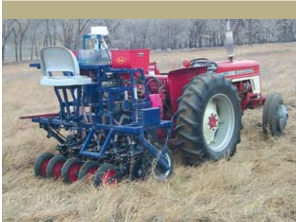
Drill seeding controls seeding rates and promotes germination by placing seeds at specific soil depths.
