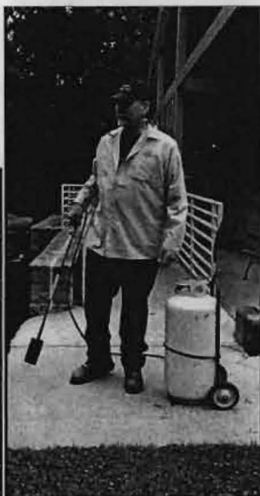
Small & Large Flamers: 30# wheeled tank and hand- held for spot treating weeds
