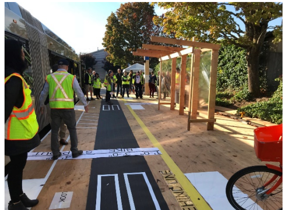
Figure 4: The City of Portland built a mock-up of a "shared platform" bus stop in a parking lot, so that staff from different City agencies and representatives of several advocacy groups, including the Oregon Commission of the Blind and Oregon Walks, could experience the design and provide feedback on how it operated before the City moved forward with constructing a shared platform stop.
