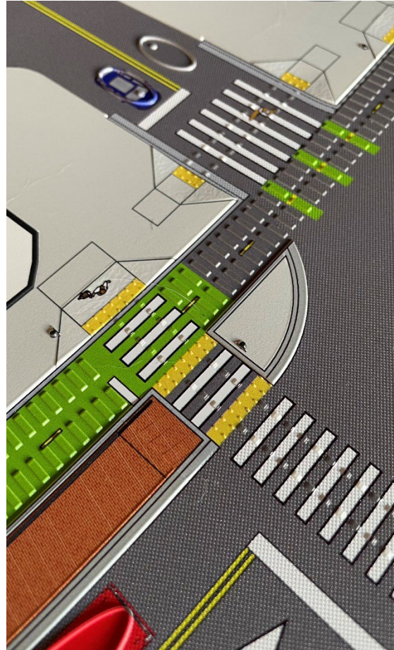
Figure 2: Tactile graphic developed for this project showing a preliminary concept for the intersection of Fenton Street and Ellsworth Drive in downtown Silver Spring.
