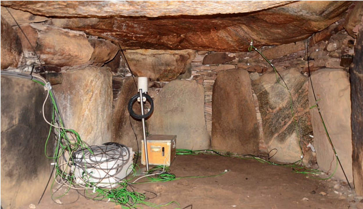
Fig. 11. The chamber in the passage grave Maglehøj with the climate monitoring equipment. Sensors for measuring temperature and humidity can be seen mounted on the surface of the stones and have been installed in the floor and in the earthen mound. Weather conditions – including precipitation – are also monitored outside the mound (photo: T. Dehn).
