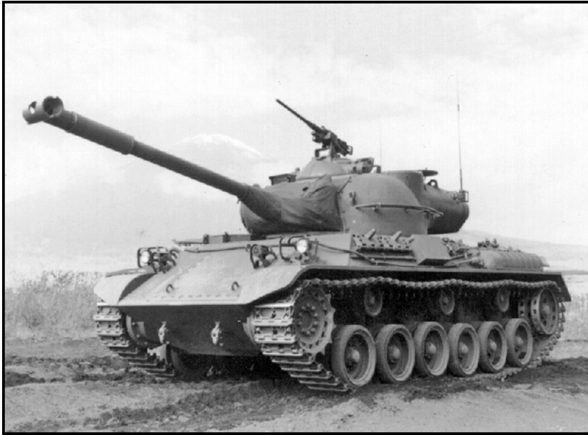
The Type 61, above, was Japan's first postwar tank design. It mounted a 90mm gun.
