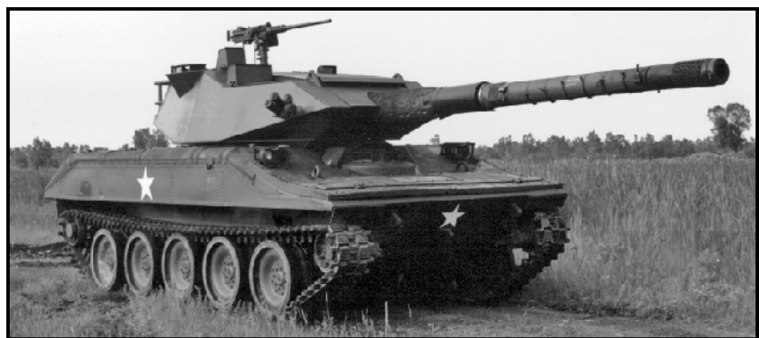
One experimental attempt to extend the Sheridan's life was this 105-mm low-recoil turret developed by Cadillac Gage.
