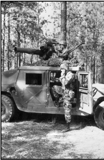
The HMMWV, shown here with TOW launcher. Would a 106mm recoilless rifle be a better armament system?
