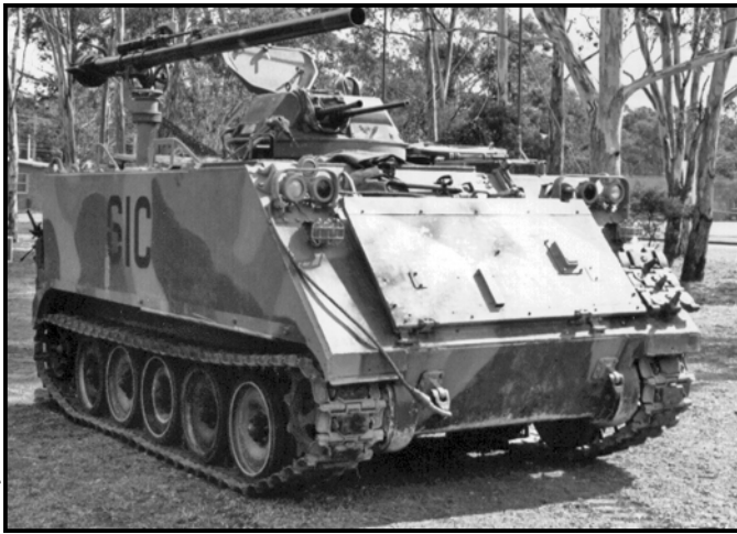
The M113-106mm RCLR solution: Unbalanced weight was a problem.
