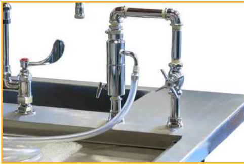
OA-510 - HYDRO-ASPIRATOR ASSEMBLY, DECK MOUNT With built-in vacuum breaker and control lever used to reverse the flow of water directing it through the hose connections for drawing fluid or rinsing.
