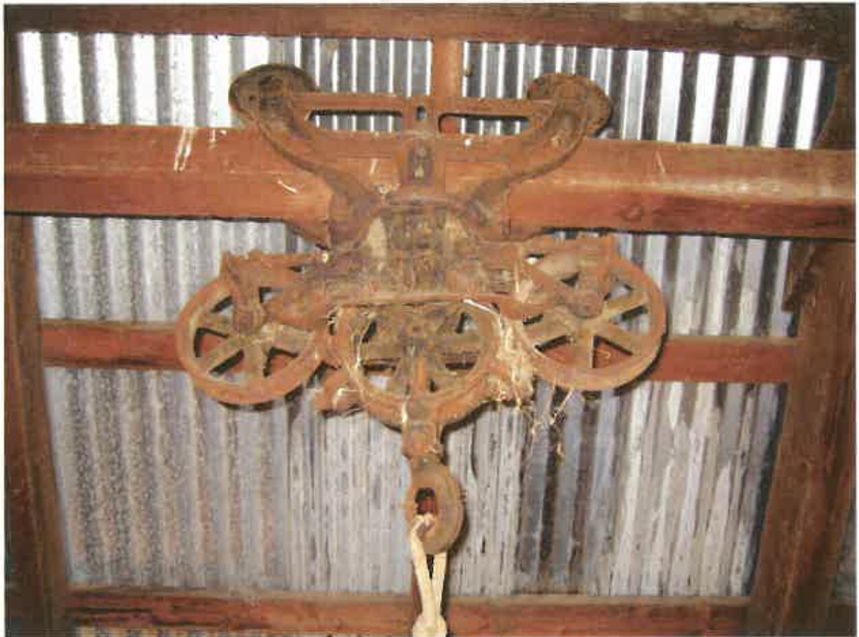
Figure 66. Hoist at the center aisle used to transfer hay in and out of the Fish Lower Barn. The hoist rides along the square beam hung from the ridge beam above.
