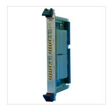
Cobalt 57670 and 58670 consist of one or two 71670 XMC modules mounted on a VPX carrier board. The 57670 is a 6U board with one 71670 module while the 58670 is a 6U board with two XMC modules rather than one.
