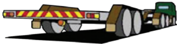
Showing typical fitting of alternative style class 2 plate (type 1)
