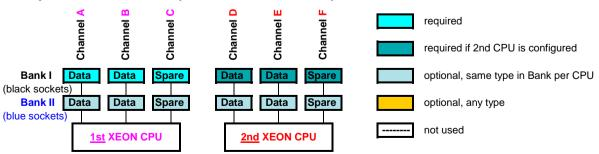
Spare Channel Mode requires identical modules on all channels of each Bank per CPU one third of the capacity is used for the spare => the available memory for applications is two thirds of the installed memory Spare Channel Mode is supported using RDIMM memory modules
