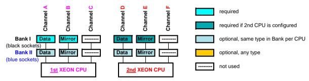
Mirrored Channel Mode requires identical modules on channel A and B (1st CPU) or channel D and E (2nd CPU) 50% of the capacity is used for the mirror => the available memory for applications is only half of the installed memory channel C (1st CPU) or channel F (2nd CPU) are not usable in Mirrored Channel Mode
