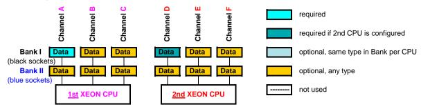
Independent Channel Mode allows all channels to be populated in any order Can run with differently rated DIMMs and use the settings of the slowest DIMM installed in the system Independent Channel Mode is supported using UDIMM or RDIMM memory modules
