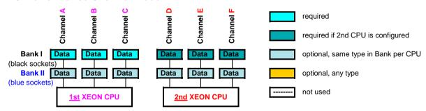
Performance Channel Mode requires identical modules on all channels of each Bank per CPU Performance Channel Mode is supported using RDIMM memory modules
