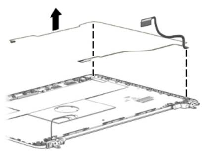
If it is necessary to replace the webcamera/microphone module or microphone module:
