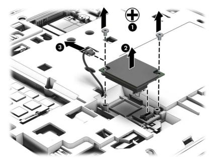
Release the modem module connector board from the clip, and then release the ZIF connector to remove modem module connector board.
