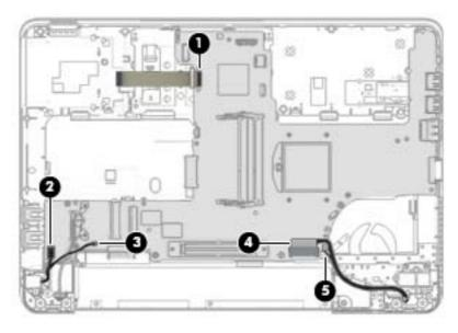
Remove the five Torx screws (1) and the Phillips screw (2) that secure the system board to the base enclosure.
