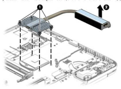
For computer models equipped with discrete graphics, following the 1 through 2 sequence stamped into the graphics board heat sink, remove the 2 captive screws (1). Following the 1 through 4 sequence stamped into the processor heat sink, loosen the four Phillips captive screws that secure the processor heat sink to the system board (2), and then remove the heat sink assembly (3).
