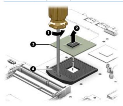
Reverse this procedure to install the processor.
