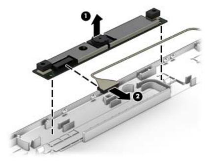
Remove the webcamera/microphone module. c.
