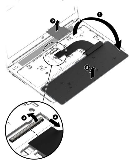
6. For models with a pointing stick, disconnect the pointing stick cable from the system board (32), release the zero insertion force (ZIF) connector to which the keyboard cable is attached (3), remove the keyboard cable (4), and then remove the keyboard (5)
