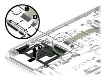
Reverse this procedure to install the smart card reader and cable.
