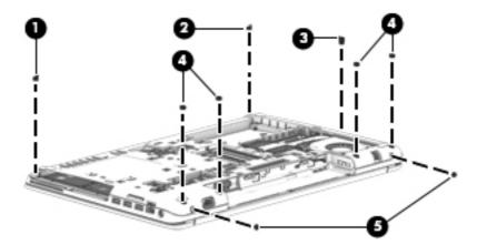
2. Remove the fourteen Torx T8 screws that secure the top cover to the computer.
