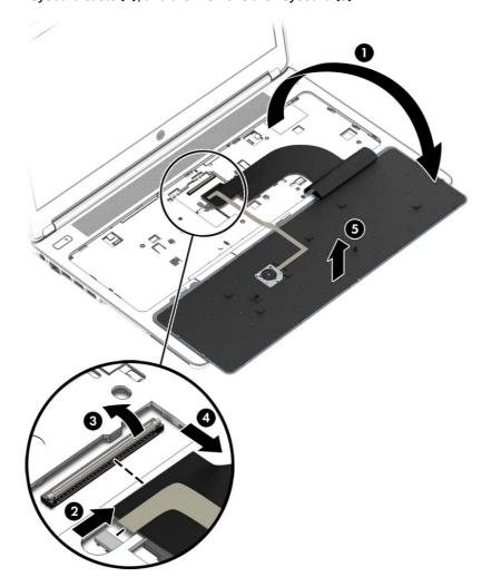
Reverse this procedure to install the keyboard.
