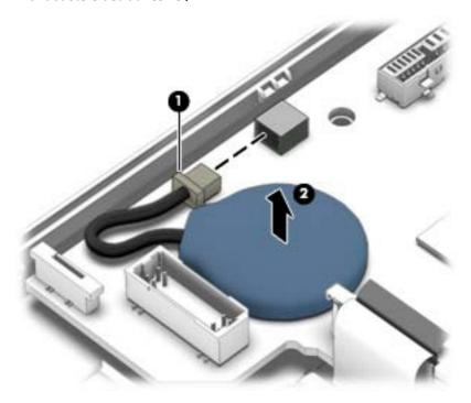
Remove the RTC battery and cable.
