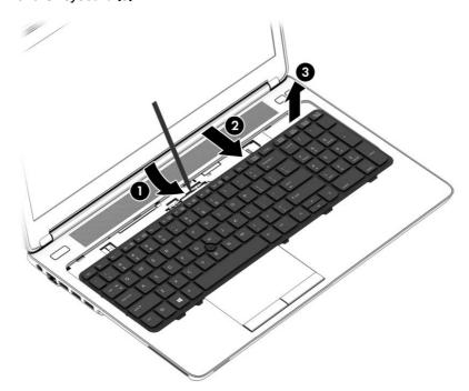
4. Swing the rear edge of the keyboard (1) up and forward until it rests upside down on the palm rest.
