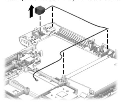
Remove the power connector cable.
