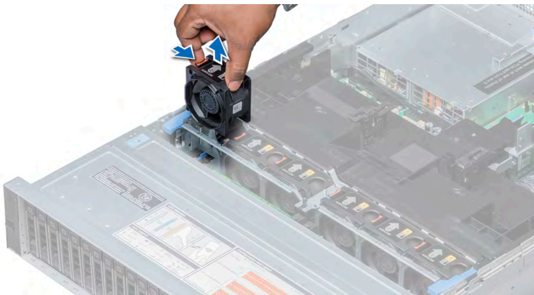
Figure 29. Removing cooling fan
