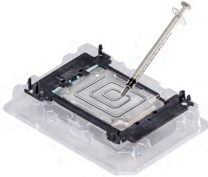
Figure 48. Applying thermal grease on top of the processor
