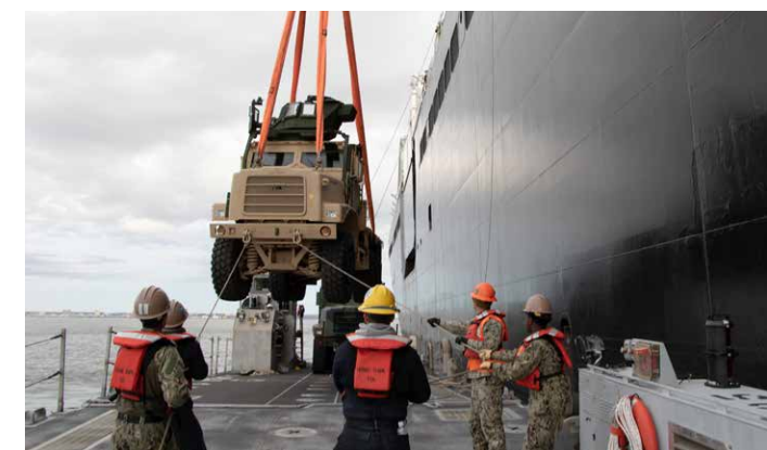
Sailors from Amphibious Construction Battalion 1 and Navy Cargo Handling Battalion 1, as part of the Navy Support Element in support of exercise Resolute Dragon 22, lower a Medium Tactical Vehicle Replacement with lines onto the deck of an Improved Navy Lighterage System craft during crane operations while moored to USNS Dahl (T-AKR 312) in Kushiro Port, Japan. (U.S. Navy photo by Mass Communication Specialist 1st Class Storm Henry)
