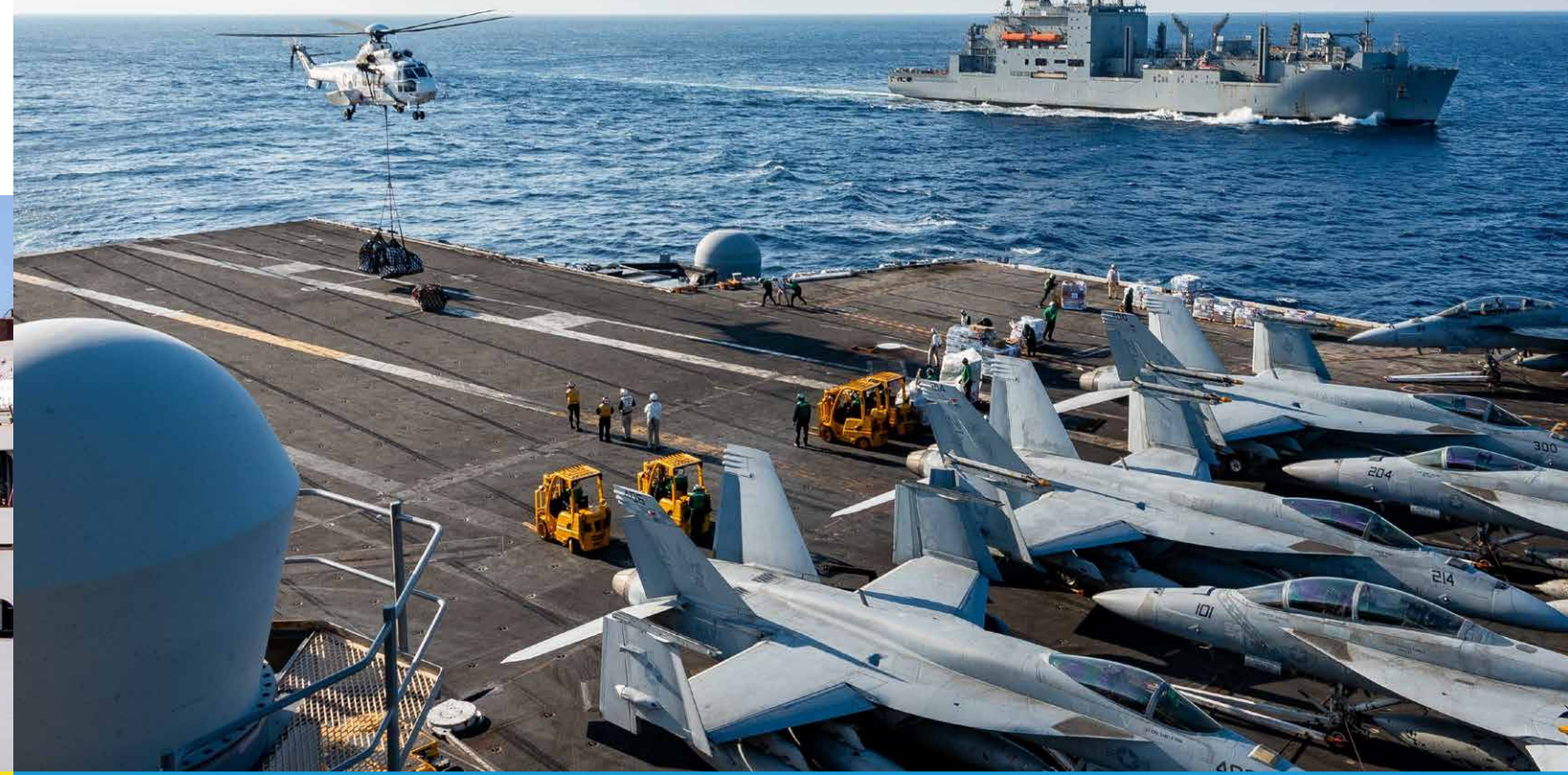
A Super Puma (EC-225) helicopter delivers cargo on the flight deck of U.S. Navy's only permanently forward-deployed aircraft carrier, USS Ronald Reagan (CVN 76), during a vertical replenishment with the dry cargo and ammunition ship USNS Charles Drew (T-AKE 10), in the Philippine Sea. (U.S. Navy photo by Mass Communication Specialist 3rd Class Oswald Felix Jr.)
