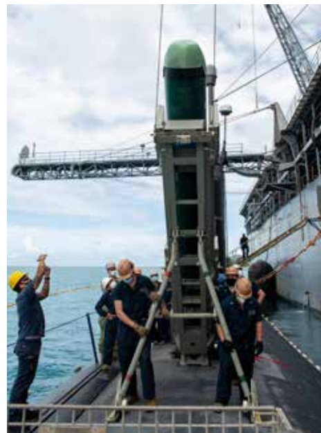
Sailors assigned to the Los Angeles-class fast attack submarine USS Hampton (SSN 767) load a MK-48 inert training shape alongside the submarine tender USS Frank Cable (AS 40) during a weapons handling exercise. (U.S. Navy photo by Mass Communication Specialist 1st Class Charlotte C. Oliver)
