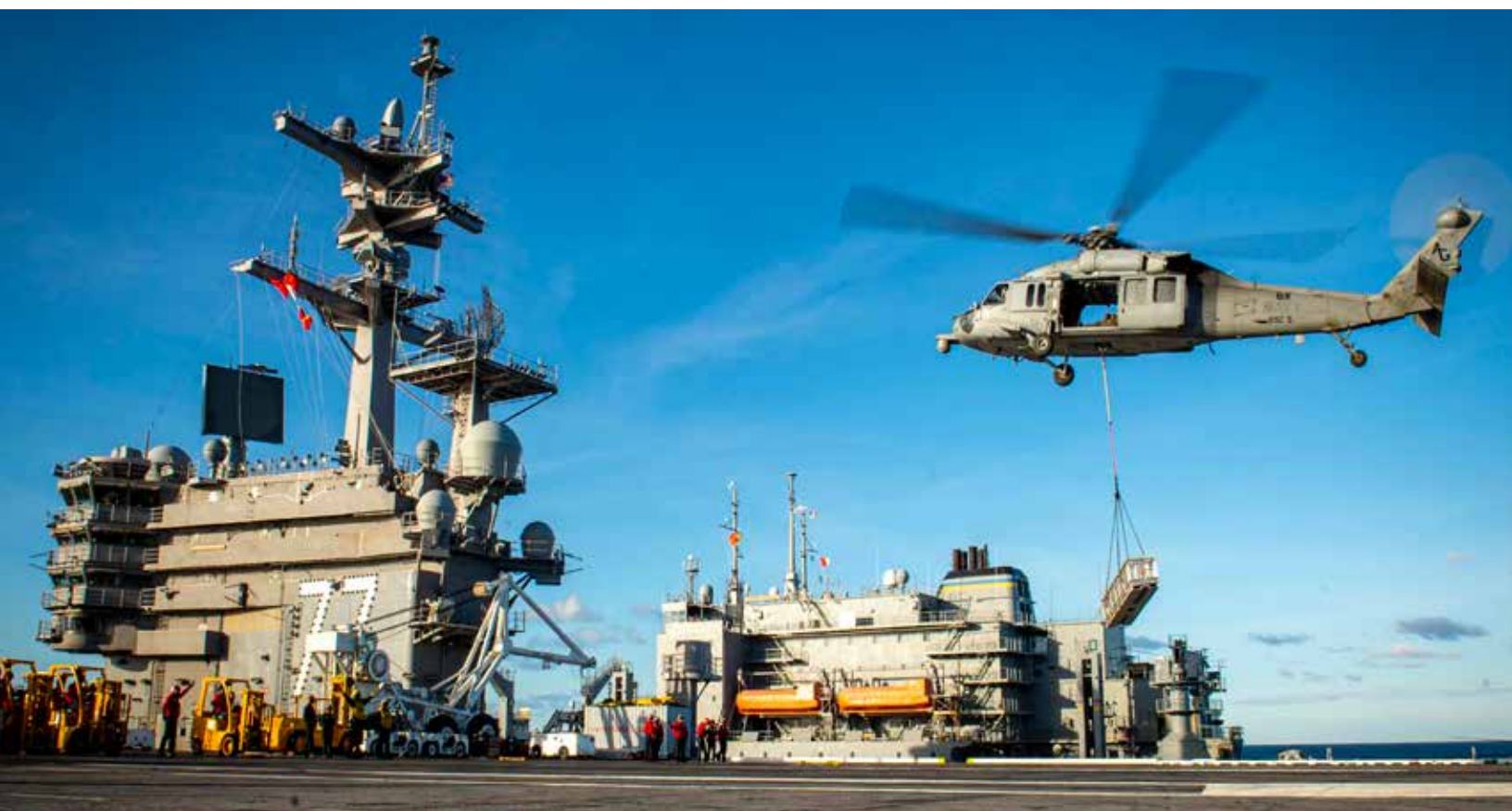
An MH-60S Sea Hawk helicopter attached to Helicopter Sea Combat Squadron 5 (HSC 5) deposits ammunition received from USNS Medgar Evers (T-AKE 13) onto the flight deck of USS George H.W. Bush (CVN 77) during a vertical replenishment. (U.S. Navy photo by Mass Communication Specialist 3rd Class Brandon Roberson)
