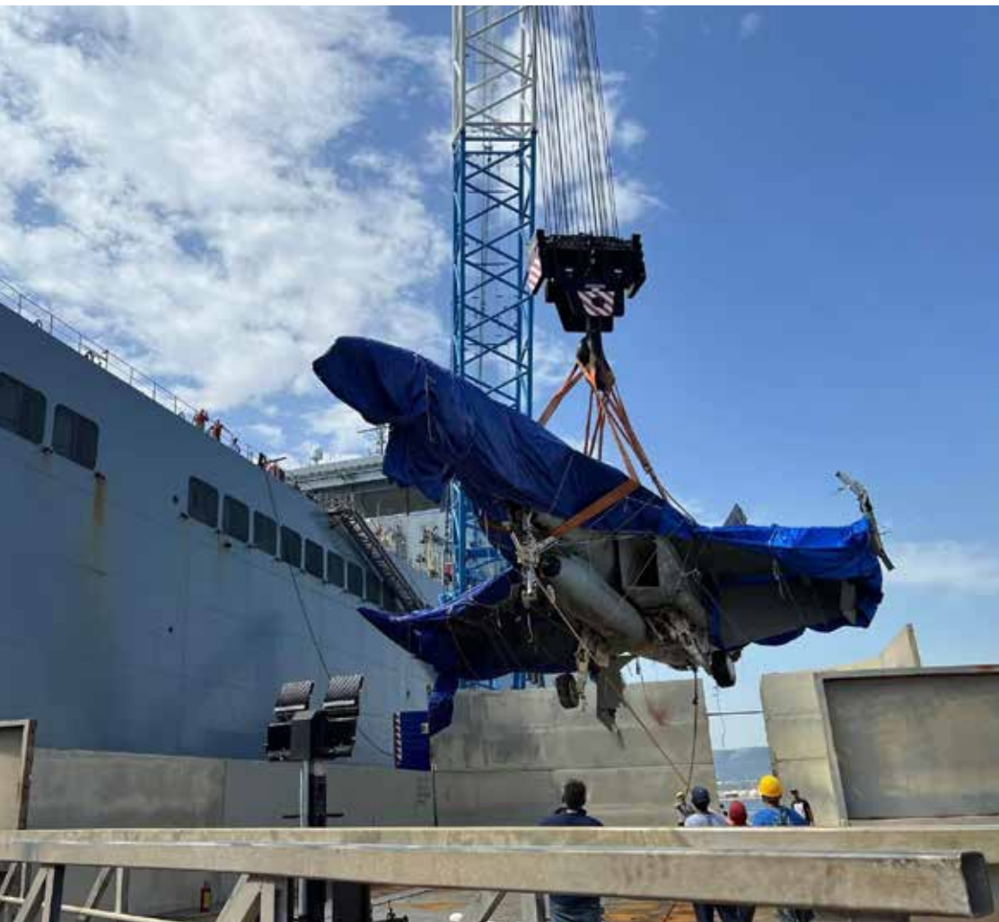
A view of an F/A-18E Super Hornet being lowered onto large, medium-speed, roll-on/roll-off ship USNS Mendonca (T-AKR 303) in Sicily, Italy. (U.S. Navy photo)
