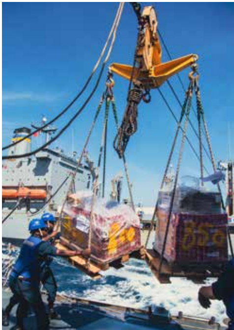
U.S. Navy Sailors direct cargo during a replenishment-at-sea (RAS) with the fleet replenishment oiler USNS John Ericsson (T-AO 194) aboard the guided-missile destroyer USS Momsen (DDG 92). (U.S. Navy photo by Mass Communication Specialist 3rd Class Lily Gebauer)
