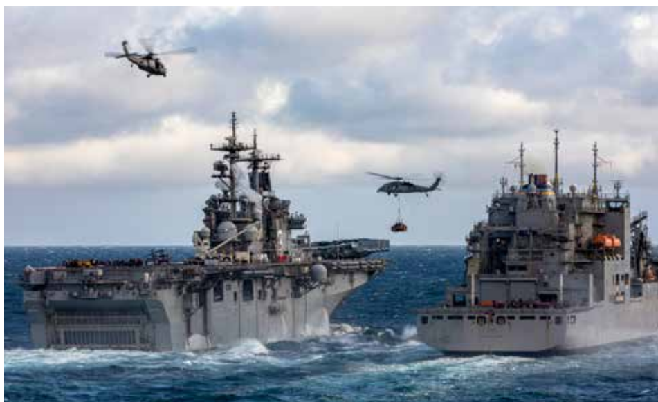
HM-60 Seahawks attached to Helicopter Squadron Command 26 and Helicopter Squadron Command 22 fly packages from the Lewis and Clark-class dry cargo ship USNS Robert E. Peary (T-AKE 5) , right, to the third Wasp-class amphibious assault ship USS Kearsarge (LHD 3), during a vertical replenishment. (U.S. Navy photo by Mass Communication Specialist Seaman Keith Nowak)
