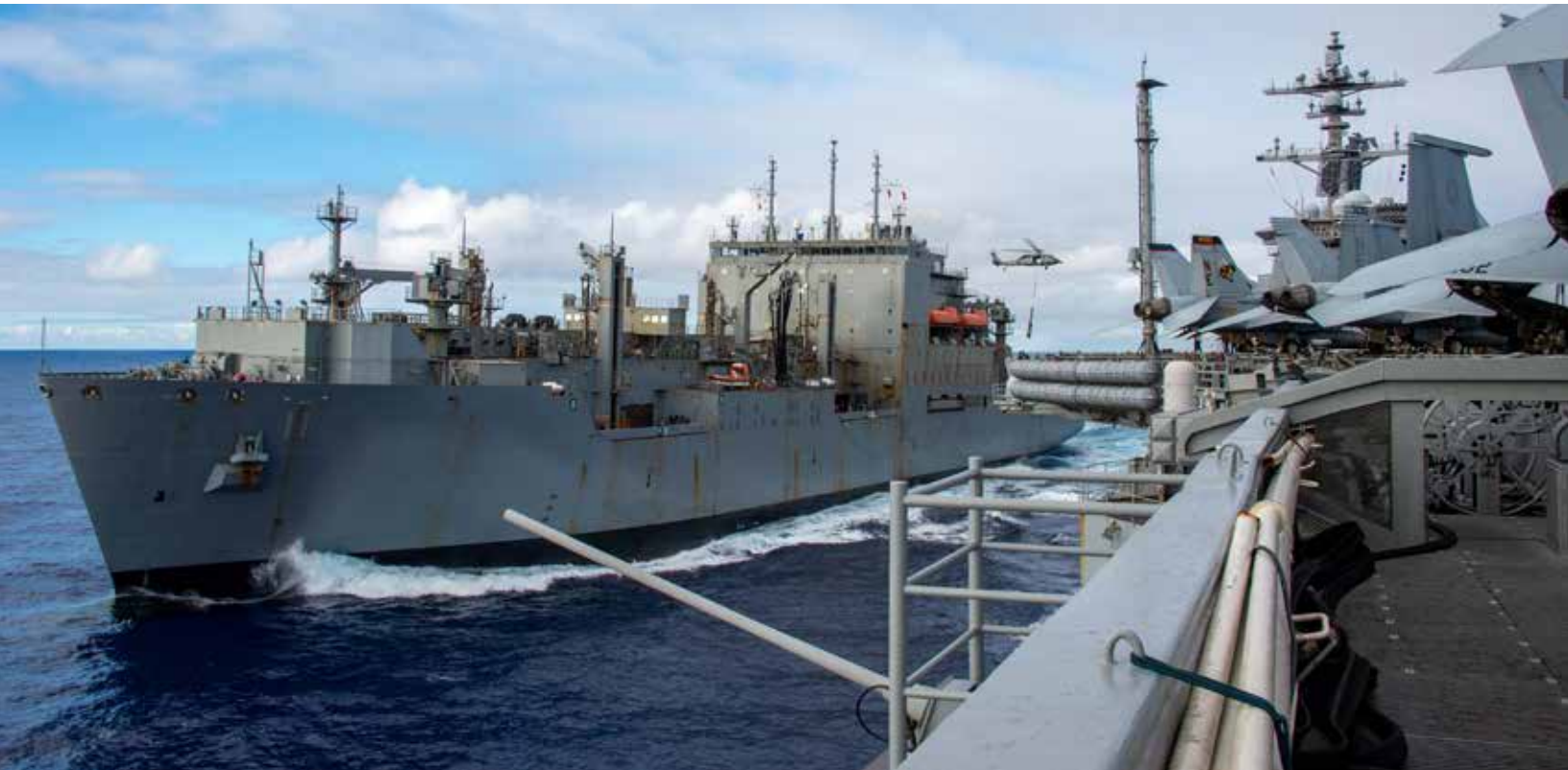
Nimitz-class aircraft carrier USS Carl Vinson (CVN 70) conducts a vertical replenishment-at-sea with Lewis and Clark-class dry cargo and ammunition ship USNS Washington Chambers (T-AKE 11) . (U.S. Navy photo by Mass Communication Specialist 3rd Class Emily Claire Bennett)
