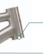
44mm Headtube Diameter: Designed for a 1.5" headset with external lower cup for a tapered fork, and a zero stack upper cup, spec'd for a 100mm tapered fork.
