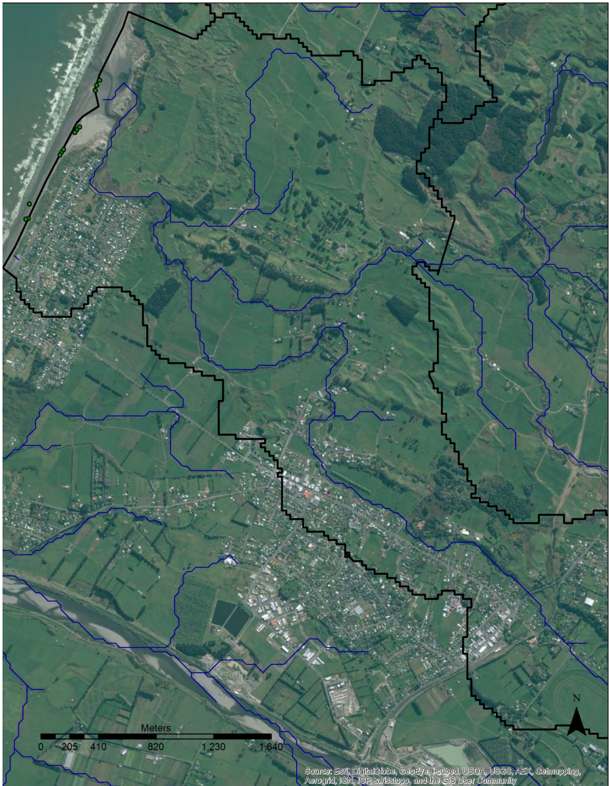
Figure A2.6b. 2008: Approximate sub-catchment feeding shallow groundwater at the Ōtaki / Waitohu tuatua sampling points (sites: north of Waitohu, south of Waitohu and Otaki, Otaki [surf club]).
