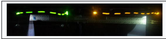
14-P12: Left trolley pushed, collides with right trolley (initially at rest)
