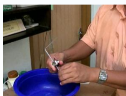
13-P2: Cutting glass tubing
