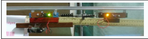
14-P11: Elastic collision between two trolleys, left trolley 3 times more massive – before collision
