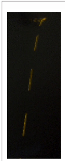
14-P17: An object falling under gravity. Its acceleration can be determined
