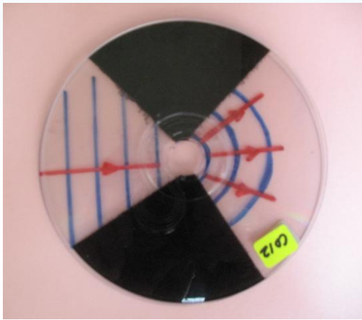
16-P7: Diffraction of Waves The two dark quadrants are rotated to reveal the wave pattern of waves after the gap
