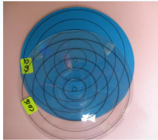
16-P8: Interference of Waves Superposition of waves of medium wavelength
