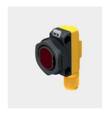
Retroreflective sensors incorporate emitter and receiver in the same housing. The light beam of the emitter is aimed at a reflector, which reflects the beam back to the receiver. An object is detected if it interrupts the light beam.
