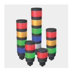
The TL50 LED tower lights indicate statuses clearly visible and permit a clear operator guidance within the entire plant. Each tower light is configured from different colored LED elements with or without a beeper and is installed ready for operation in a few handling steps. The LED elements and their flashing frequency, as well as the beeper can be individually controlled via IO-Link.
