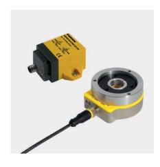
The contactless operating encoder Ri-QR24 makes no compromise in terms of robustness and tightness. A mechanical coupling between the sensor and the machine shaft is – in contrast to conventional rotary encoders – no longer required. With IO-Link the measuring signal can be inexpensively and effectively evaluated and also the zero point of a measurement set.
