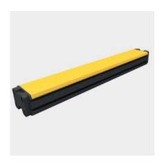
The inductive linear position sensors operate without contact and wear-free thanks to a revolutionary measuring principle. The position is not detected via a positioning magnet but via an oscillating RLC circuit. IO-Link is used, in addition to the digital transmission of process data, also for application-specific adaptation, for example by setting the measuring range.
