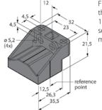
Floating positioning element for Li-Q25L; the nominal distance to the sensor is 1.5 mm; pairing with the linear position sensor at a distance of up to 5 mm or misalignment tolerance of up to 4 mm.
