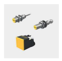
With uprox®3 IO-Link Turck offers the factor 1 sensors now also with IO-Link interface. The flexibility thus obtained makes the uprox®3 IO-Link sensor the "Swiss army knife" of factor 1 sensors. The range of functions include adjustable switching outputs, different output functions (PNP/NPN, NO/NC), various speed monitoring functions and advanced sensor data such as the internal sensor temperature or sensor ID data.
