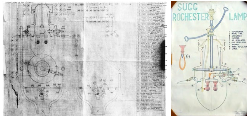
14a 來自原供應商的檔案資料庫「羅車士打款式」煤氣路燈的製作平面圖及手繪圖 Plan and drawing of the “Rochester Lamp” from the archives of the original supplier
