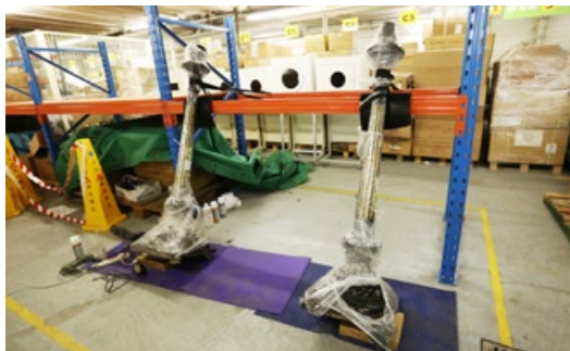
13 專門承辦商在煤氣公司的倉庫為兩支鑄鐵燈柱進行非破壞性測試 A specialist contractor conducted a non-destructive test on the two cast-iron columns at the Towngas store.
