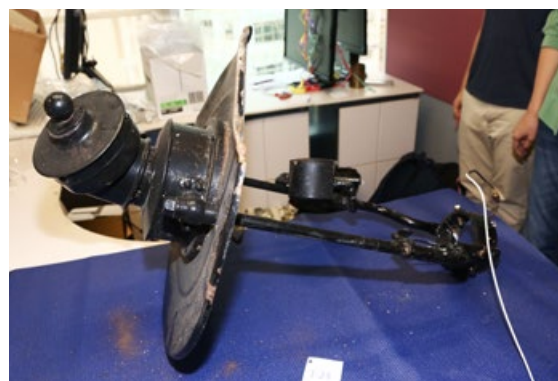
7 其中一盞嚴重變形的燈頭 One of the seriously deformed gas lanterns
