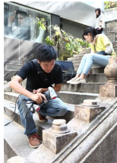
19 古蹟損毀後，古蹟辦三維掃描小組到現場使用座地式激光掃描儀（左）及手提式三維激光掃描儀（右）進行三維掃描。 After the damage, 3DSU of AMO conducted 3D scanning on-site using both the terrestrial laser scanner (left) and the portable 3D scanner (right).
