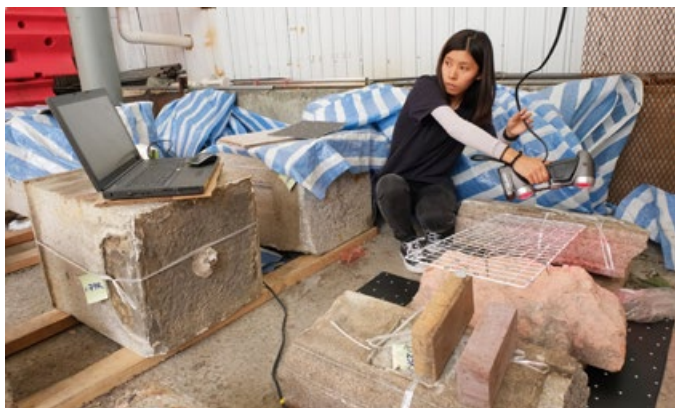
20 三維掃描小組以手提式三維激光掃描儀為花崗石碎片進行掃描，以便取得碎片形狀及尺寸的準確資料。 The broken granite fragments were scanned by 3DSU using the portable 3D scanner to acquire accurate data for their shapes and dimensions.
