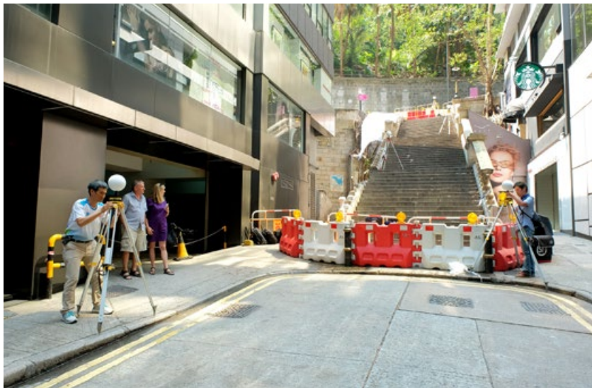
19 古蹟損毀後，古蹟辦三維掃描小組到現場使用座地式激光掃描儀（左）及手提式三維激光掃描儀（右）進行三維掃描。 After the damage, 3DSU of AMO conducted 3D scanning on-site using both the terrestrial laser scanner (left) and the portable 3D scanner (right).
