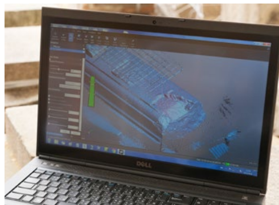
20 三維掃描小組以手提式三維激光掃描儀為花崗石碎片進行掃描，以便取得碎片形狀及尺寸的準確資料。 The broken granite fragments were scanned by 3DSU using the portable 3D scanner to acquire accurate data for their shapes and dimensions.
