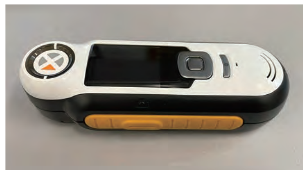
17 利用便攜式色度計進行色彩監測 (型號: X-rite RM200QC) Portable colorimeter used for the monitoring programme (Model: X-rite RM200QC)
