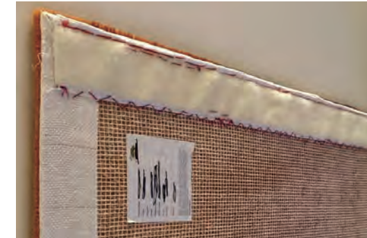
5 地氈樣本背面縫紉了 Velcro® 「環」帶 Reverse side of the sample carpet showing the sewing of the loop-side Velcro®
