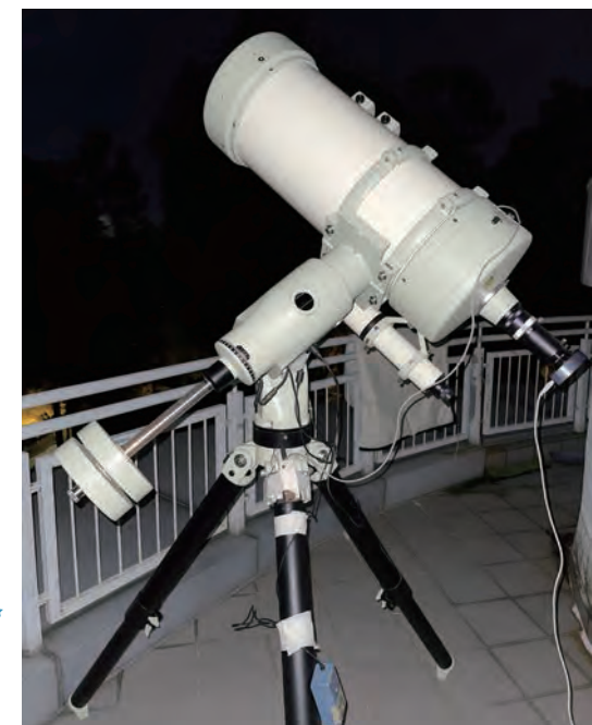
5 拍攝 QSME 的器材：300 毫米口徑的反射式望遠鏡搭載天文專用 CCD 相機。地點為香港太空館西貢遙控天文台。 The equipment for recording QSME: an astronomical CCD camera attached to a 300-mm reflecting telescope. It took place at the HKSpM's Sai Kung iObservatory.
