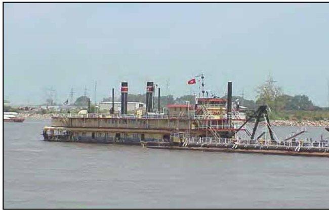
Photograph 7-19. Dredge Using Hydraulic Pipeline
