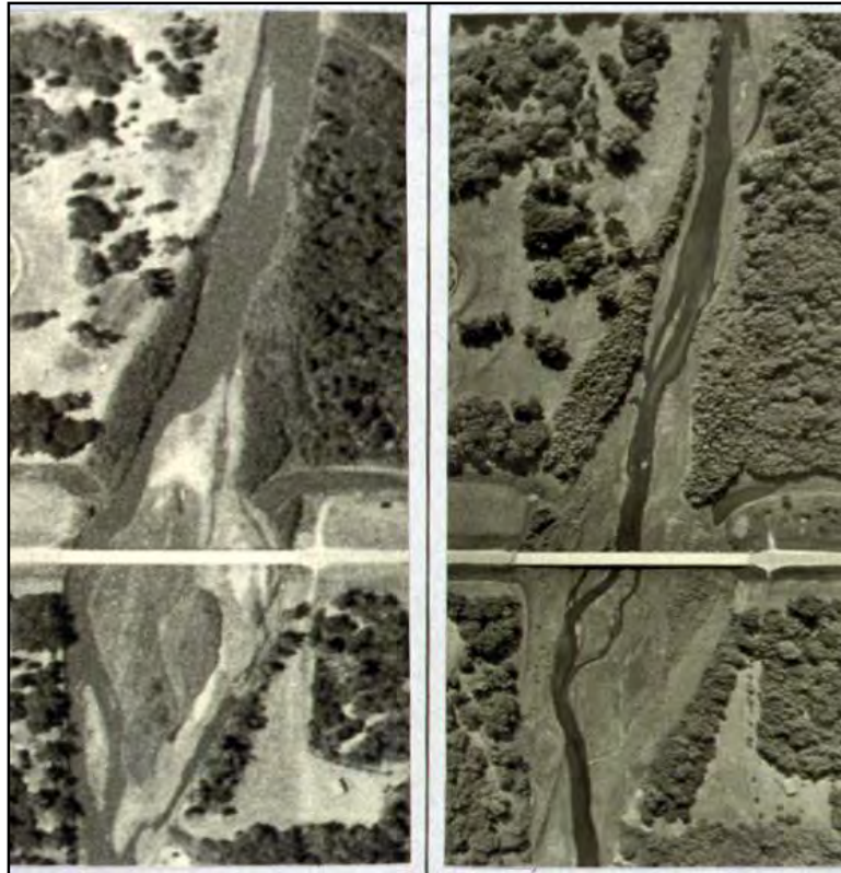
Photograph 7-15. Aerial Photograph of West Fork Cedar River (Iowa) Bridge Crossing (Left) Prior to Vane Installation in 1984, and (Right) in 1989, Five Years after Vane Installation
