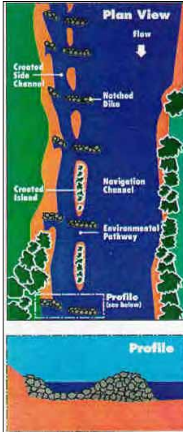
Figure 7-1. Wing Dam Notching
