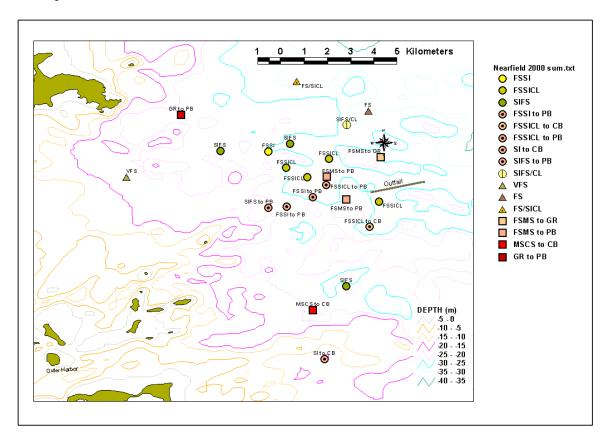
Figure 3-3. Distribution of estimated sediment types at nearfield stations based on SPI, August 2000.
