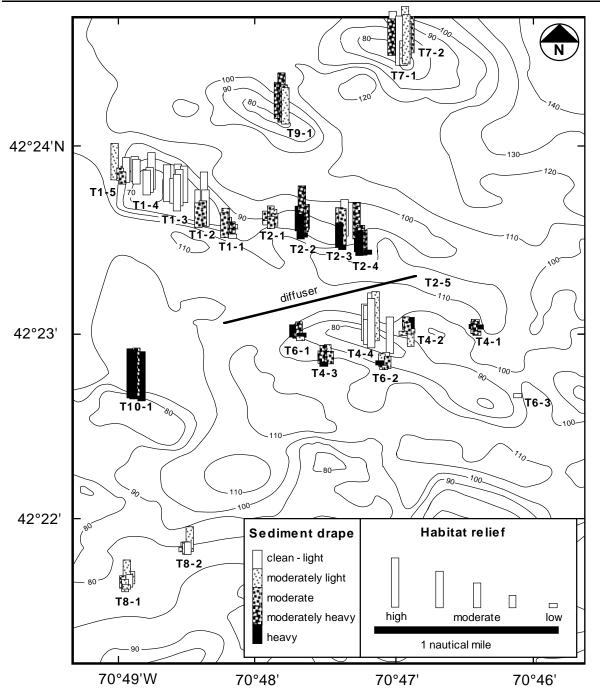
Figure 6-5. Sea floor characteristics, habitat relief and sediment drape determined from the 1995 to 2000 nearfield hardbottom surveys.
