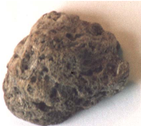
Figure 3.20: Photograph of the whitish grey pumice from Trandvikan. The pumice is about 3.5 cm in diameter. The pumice is whiter than it appears on the photograph.
