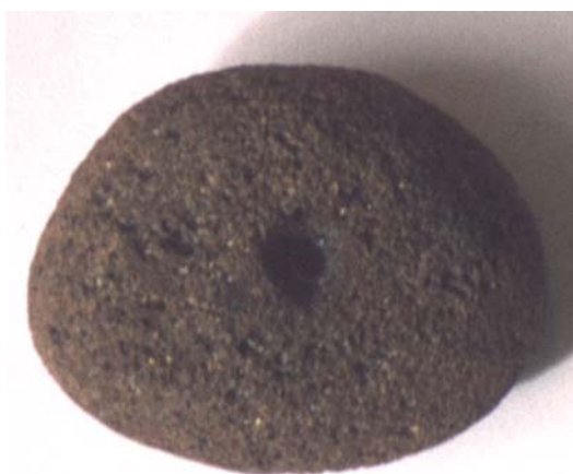
Figure 4.2: Photograph to show the oldest pumice piece U24007 (U 1) from The Udal. This is physically a typical piece of brown dacitic pumice. The hole in the pumice was created by sampling for EPMA.
