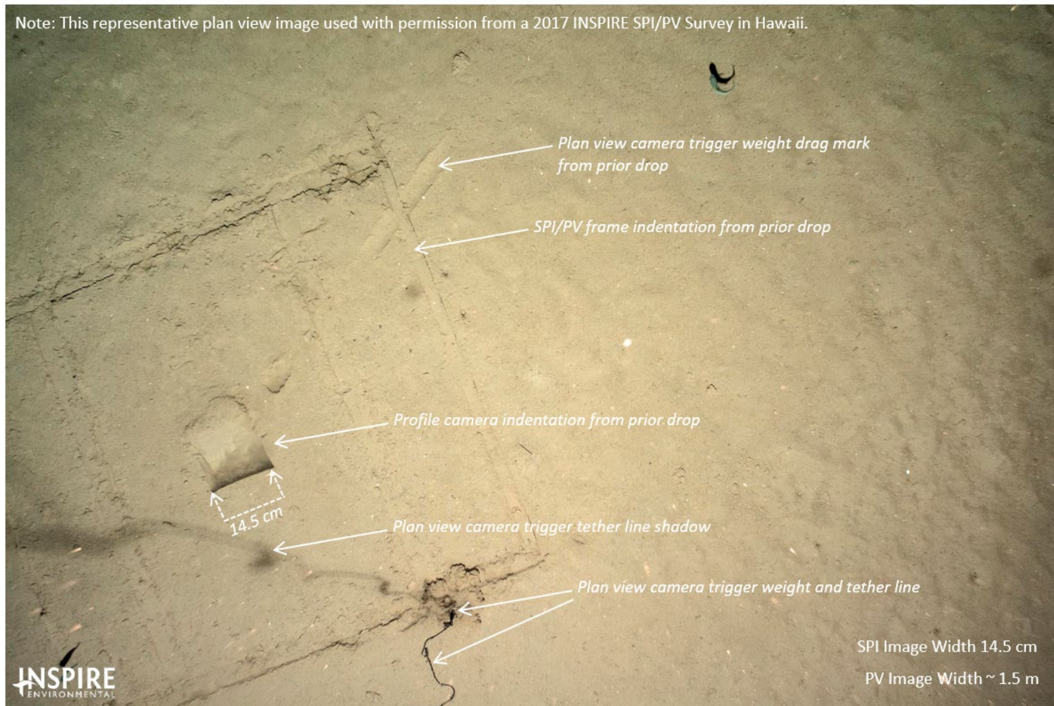
Figure 2-5. This representative plan view image shows the sampling relationship between plan view and sediment profile images. Note: plan view images differ between surveys and stations and the area covered by each plan view image may vary slightly between images and stations.
