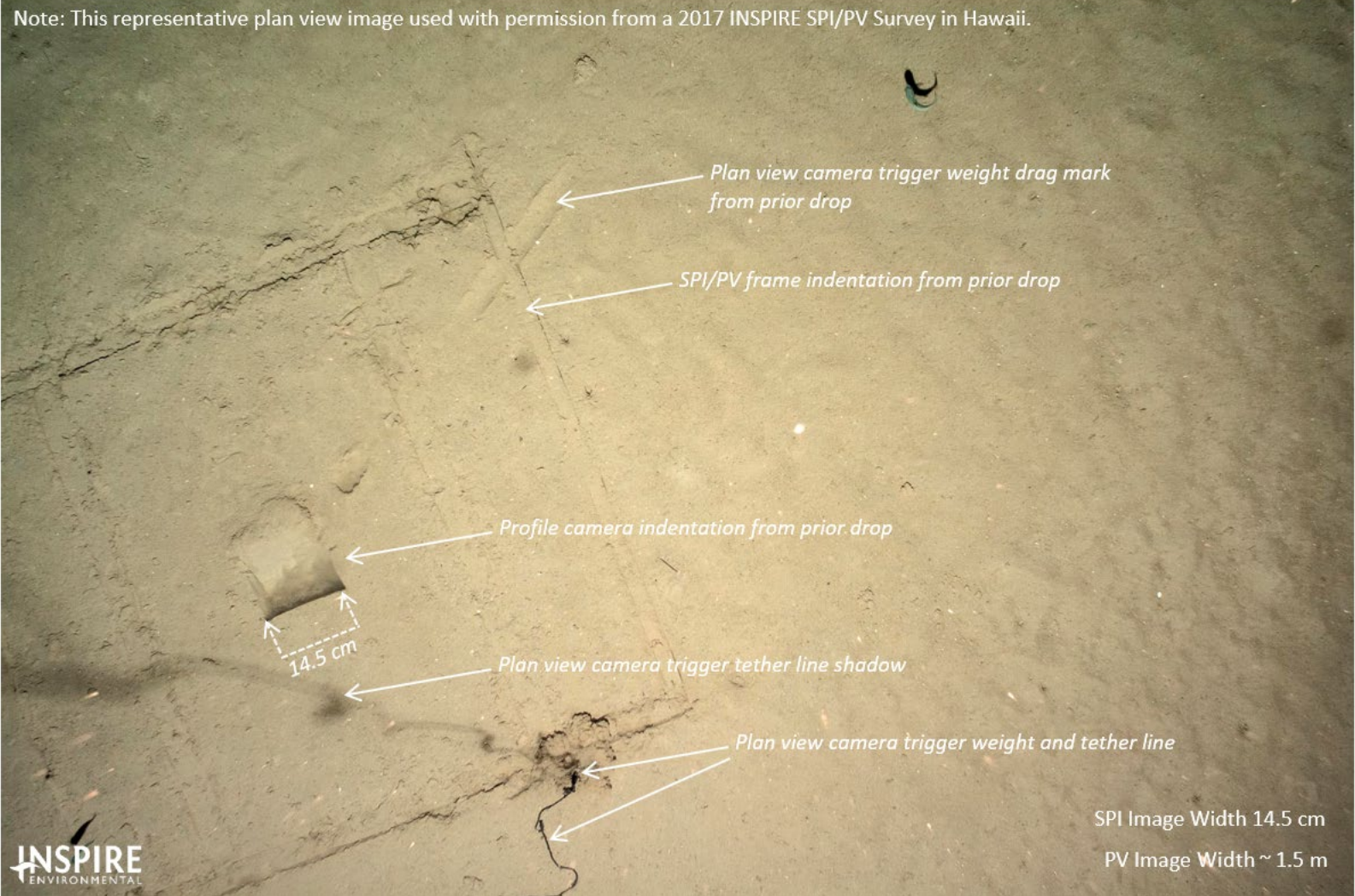
Figure 2-6. This representative plan view image shows the sampling relationship between plan view and sediment profile images. Note: plan view images differ between surveys and stations and the area covered by each plan view image may vary slightly between images and stations.
