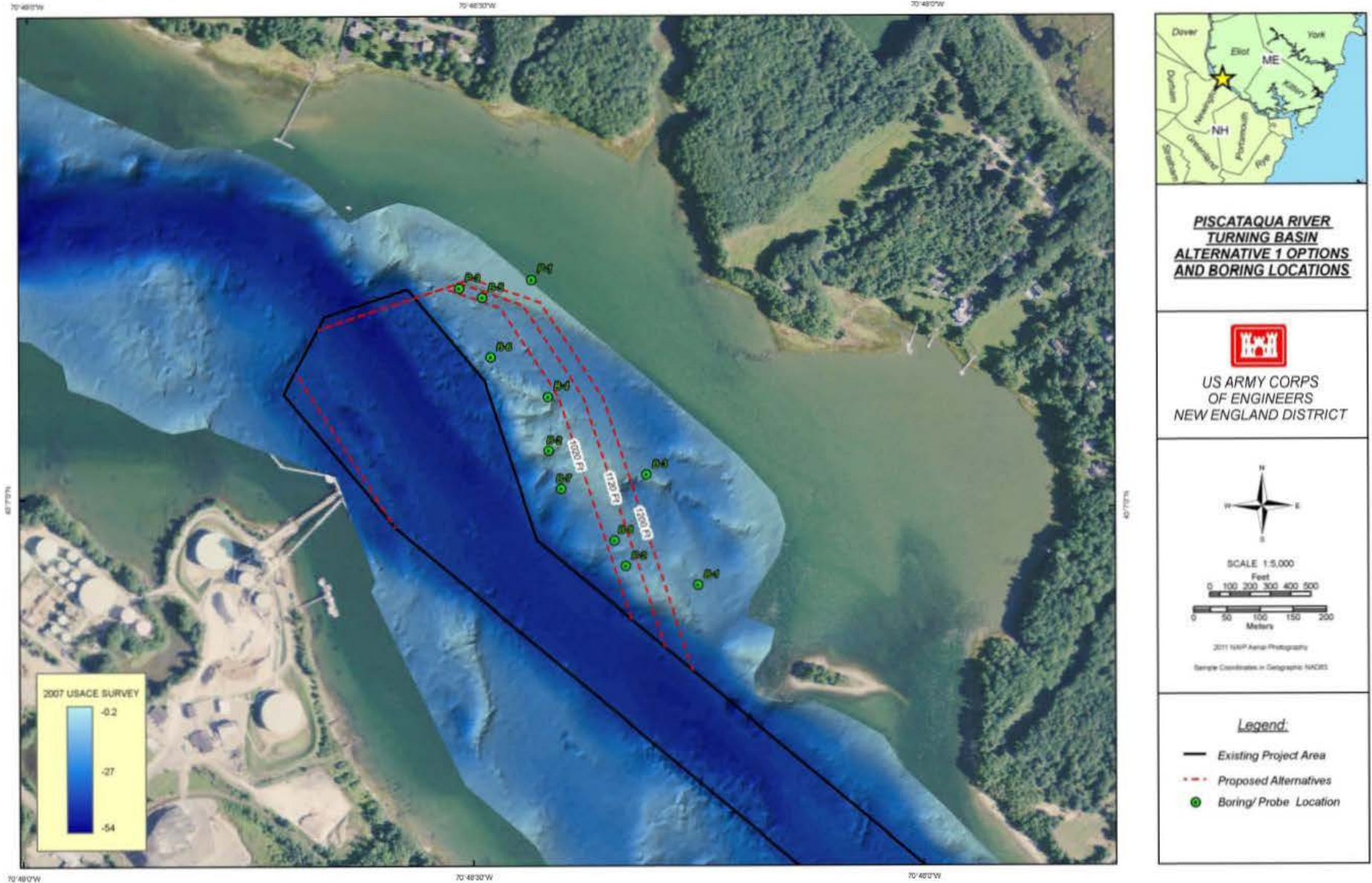
Figure 1 - Location of Borings and Probes in Upper Turning Basin Expansion Area
