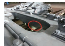
Spot where cracking is occurring on train car
