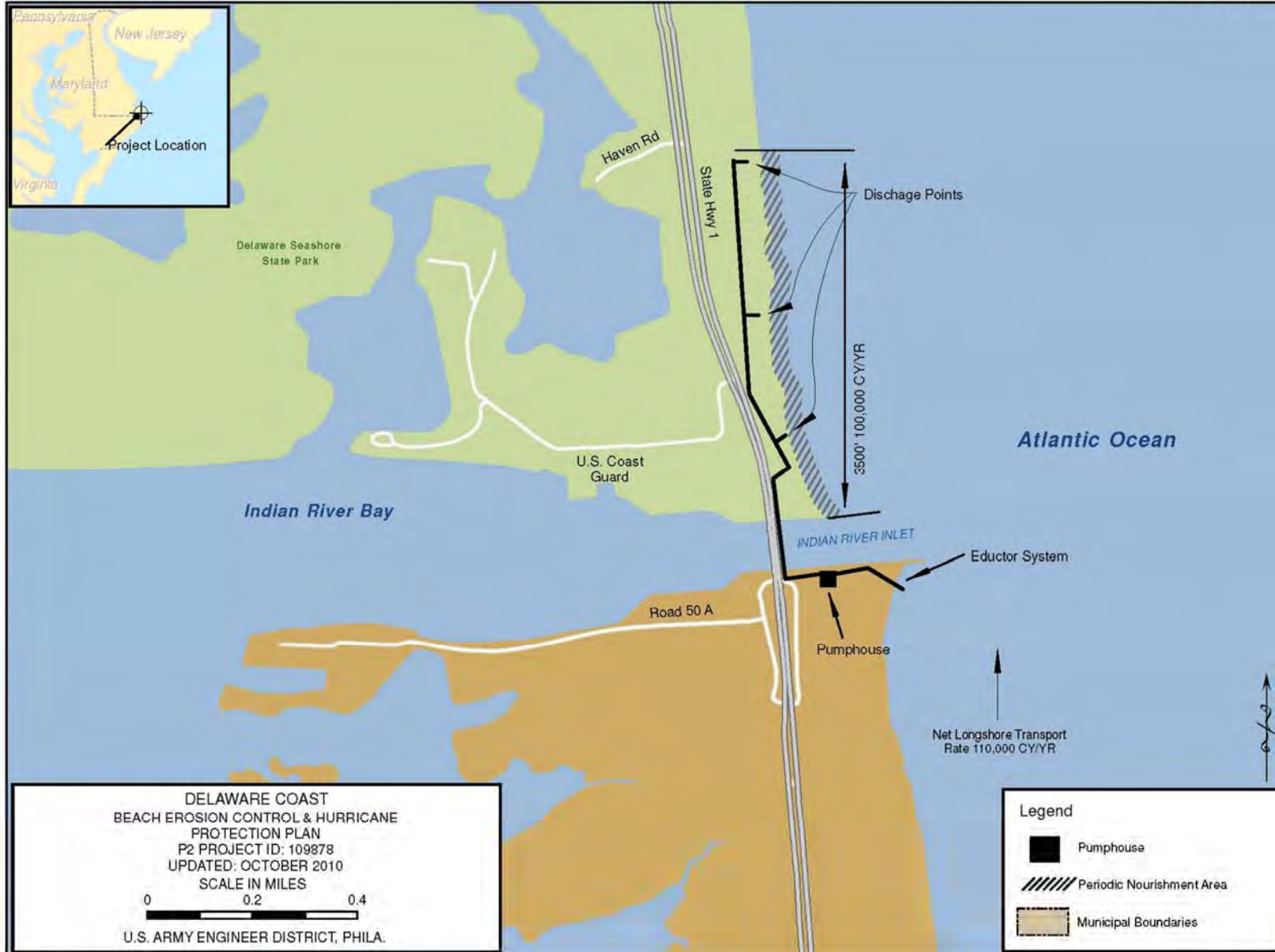
Figure 1-5. Indian River Inlet Sand bypass Project Plan.
