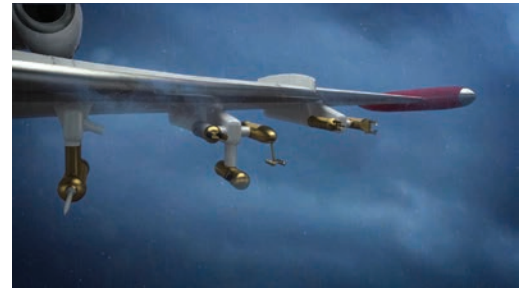
More than 20 meteorological instruments outside and inside the Gulfstream aircraft will be used to collect data on engine-icing conditions.
