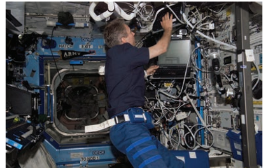
European Space Agency astronaut Thomas Reiter, Expedition 13's flight engineer, prepares the HRF-2 rack for an upgrade of the Pulmonary Function System experiment in the Destiny Laboratory of the International Space Station.
