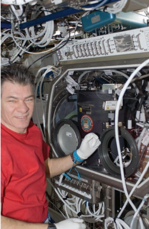
European Space Agency astronaut Paolo Nespoli, Expedition 27's flight engineer, works with the Microgravity Science Glovebox in the Destiny Laboratory of the International Space Station.
