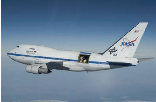
With the large door over its 2.5-meter, German-built telescope wide open, NASA's Stratospheric Observatory for Infrared Astronomy 747SP aircraft soars over southern California's high desert.
