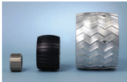
This image shows the increasing wheel size among the Mars explorers: Mars Pathfinder (left), Mars Exploration Rover (center), and Mars Science Laboratory (right).
