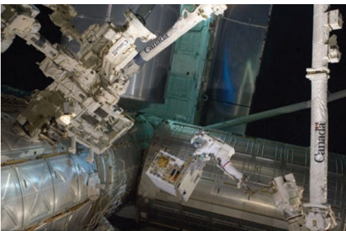
Spacewalker Mike Fossum, while anchored to the Canadian Space Agency's Dextre robot, carries the RRM module from the Atlantis cargo bay to a temporary platform on the International Space Station.
