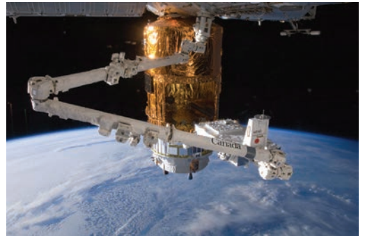
In the grasp of the ISS robotic Canadarm2, the H-II Transfer Vehicle 3 (HTV-3) Exposed Pallet is moved for installation on the Japan Aerospace Exploration Agency (JAXA) HTV-3 while it is docked to the Space Station in July 2012.
