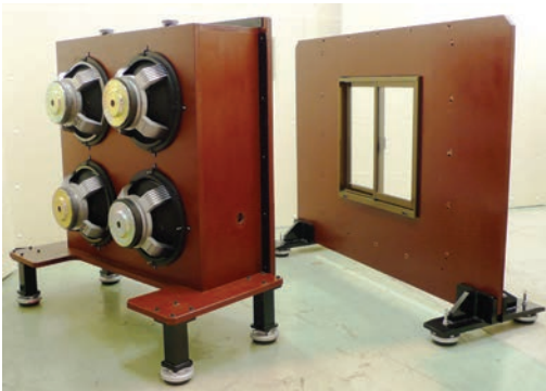
The Vibro-Acoustic Device is used in the NASA-JAXA sonic boom research testing.
