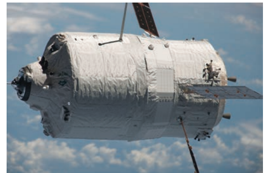
The European Space Agency's "Edoardo Amaldi" Automated Transfer Vehicle-3 (ATV-3) approaches the International Space Station in March 2012. With a successful docking, the unmanned cargo spacecraft delivers 220 pounds of oxygen, 628 pounds of water, 4.5 tons of propellant, and nearly 2.5 tons of dry cargo, including experiment hardware, spare parts, food, and clothing.
