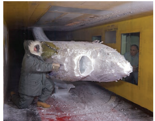
A commuter transport engine undergoes testing in the Icing Research Tunnel at the NASA Glenn Research Center.
