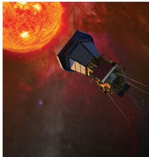
The solar panels of the Solar Probe Plus spacecraft are folded into the shadow of its protective shield as the probe gathers data on its approach to the Sun. (Credit: Johns Hopkins University Applied Physics Laboratory)
