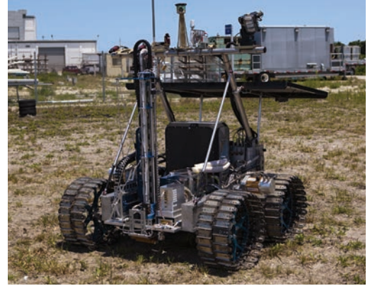
The Resource Prospector Mission is a miniature drilling and chemistry plant packaged onto a medium-sized rover to collect and analyze volatiles in lunar regolith.
