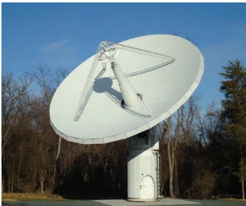
This 12-meter antenna is part of the next-generation geodetic Very Long Baseline Interferometry system at NASA's Goddard Geophysical and Astronomical Observatory in Greenbelt, Maryland. Essential new features include the fast antenna, broadband receiver, and high-rate recording at four settable bands.
