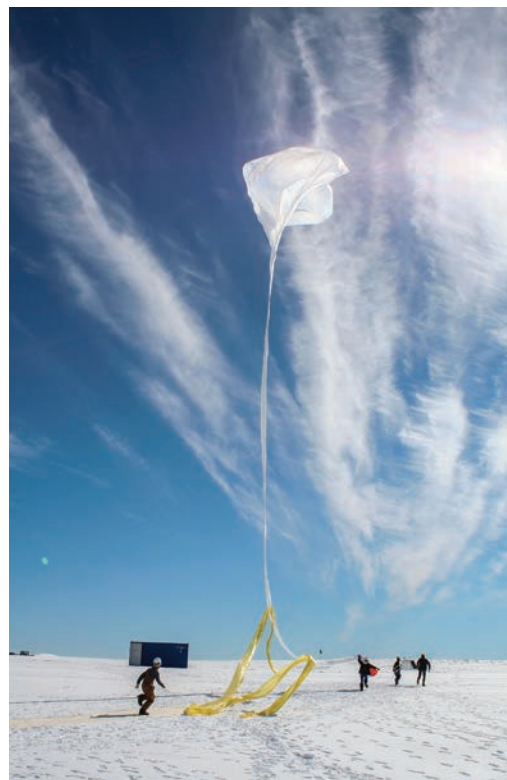
Scientists race through the Antarctic snow to launch 1 of 20 balloons as part of NASA's Balloon Array for Radiation belt Relativistic Electron Losses (BARREL) mission. Each balloon is equipped with instruments to help track how electrons from giant radiation belts surrounding Earth travel down magnetic field lines toward the poles. BARREL works in conjunction with NASA's Van Allen Probes.
