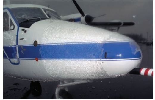
This post-flight image shows ice contamination as a result of encountering Supercooled Large Droplet (SLD) conditions near Parkersburg, West Virginia.
