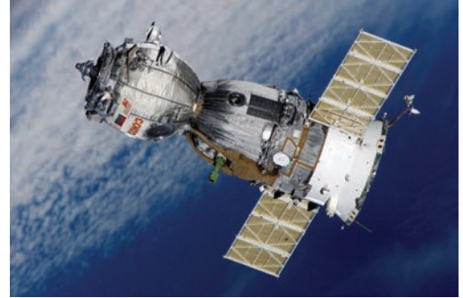
Soyuz TMA-7 orbiting Earth. The Soyuz is a crew transportation and rescue vehicle and can support up to three crewmembers.
