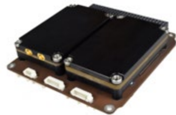
Figure 9.5: Example of software defined radio, tunable in the range 70 MHz to 6 GHz. Credit: GomSpace.
