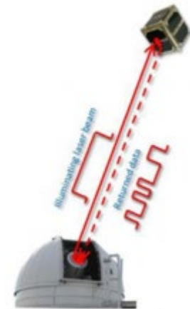
Figure 9.9: Scheme for using land-based laser to transmit data from CubeSat using on-board MRR. Credit: Salas et al. (2012).
