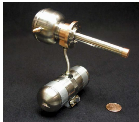
Figure 7.18: TRL6 Microcryocooler. Cryocooler Credit: Lockheed Martin.
