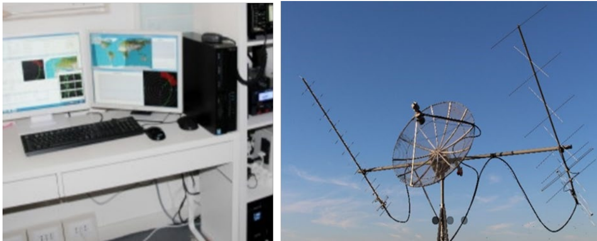
Figure 11.22: (left) GAUSS ground station hardware, transceiver and (right) tracking antenna. Credit: GAUSS Srl.
