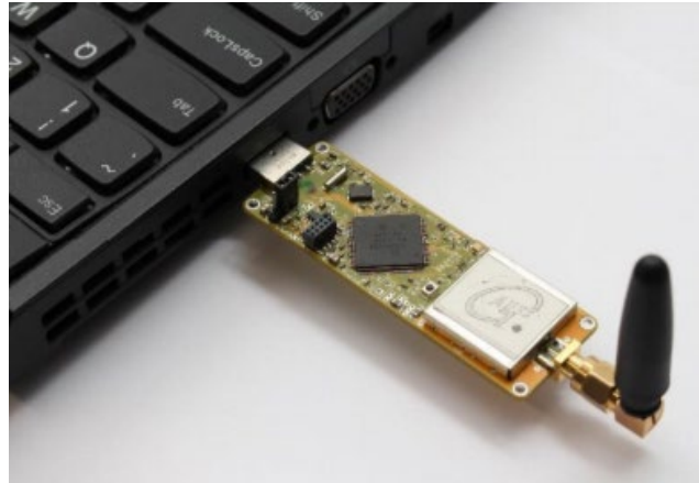
Figure 11.29: GAUSS UHF USB Mini Ground Dongle. Credit: GAUSS.
