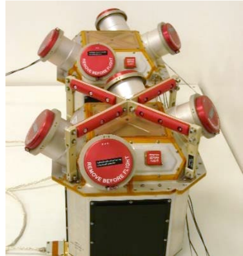
Figure 4.24: Flight CMNT modules for LISA Pathfinder. Credit: Busek.
