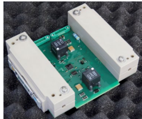
Figure 4.49: Plasma Brake Module (PBM) demo unit. Credit: Aurora Propulsion Technologies.
