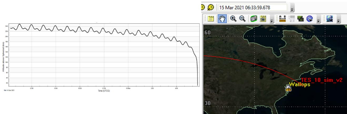
Figure 13.10: Targeting of the TES 10 Exo-brake is achieved by modifying the drag area of the modulating Exo-brake. (Left) the plot includes actual GPS readings and the approximate ballistic coefficient achieved at different parts of the mission. Credit: Jose Alvarellos et al 2021. (Right) the simulated reentry location of TES 10. Credit: Sanny Omar. The spacecraft overshot but still demonstrated the capability to target a particular location by modifying its ballistic coefficient. Credit: NASA.
