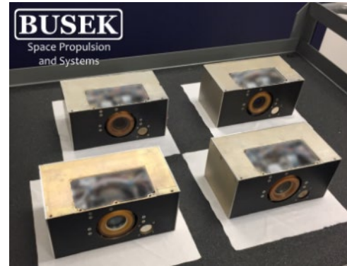
Figure 4.34: BIT-3 thruster. Credit: Busek.
