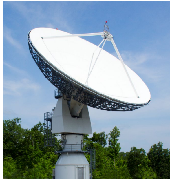
Figure 11.19: The Morehead State University 21-meter Ground Station has been upgraded with support from NASA’s Advanced Exploration Systems, to become the first non-NASA affiliated node on the DSN. Referred to as DSS-17, the station will support NASA Interplanetary CubeSat missions. Credit: Morehead State University.
