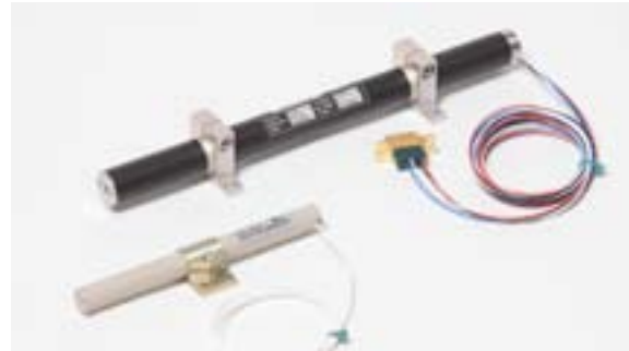
Figure 5.3: Magnatorquers for micro satellites. Credit: ZARM Technik.
