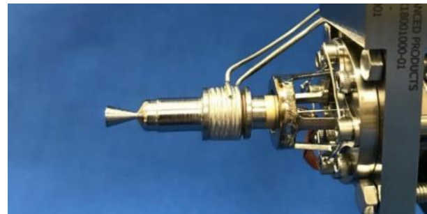
Figure 4.5: Plasma Processes LLC 100mN thruster. Credit: NASA MSFC.
