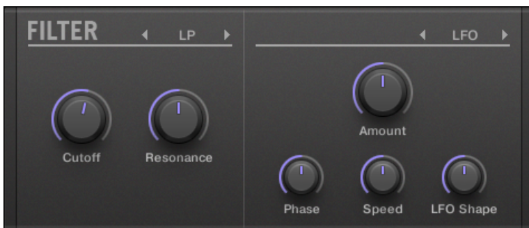
The Filter panel in the Plug-in Strip.
