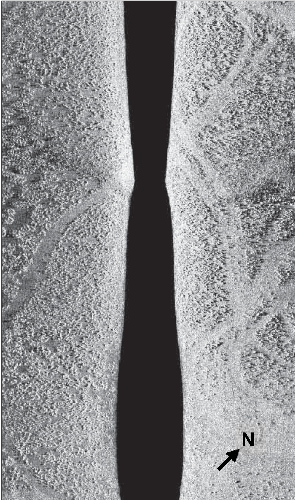
Figure 24 Non-georectified sidescan image of apparent dredge tracks through serpulid reefs off Rubha Mór in 2005. The position of the centre of the image is approximately 56.51298°N 5.38225°W. Image width 70m, length 228m
