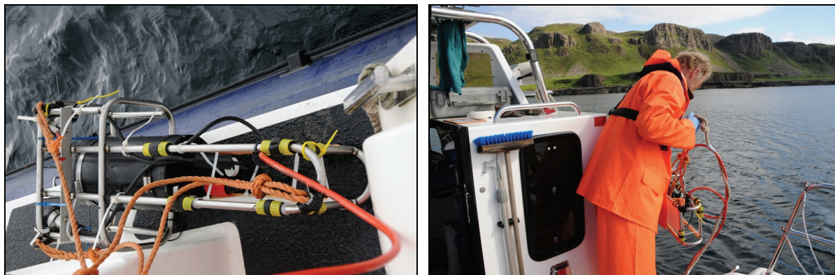
Plate 2 ASML drop camera and frame and hand deployment over the side of survey vessel Lophelia within the Sound of Canna
