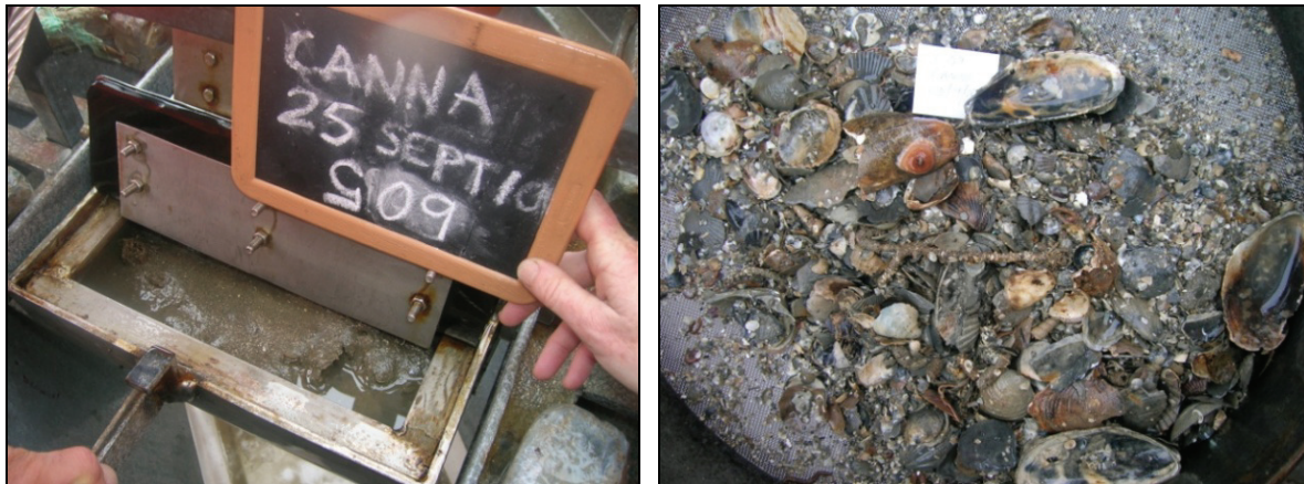
Plate 4 Example photographs showing the volume and contents of a successful grab sample (Station G09) and the residue retained in the 1 mm sieve
