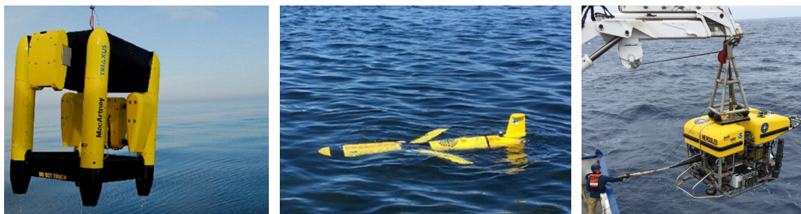
Figure 22: Images of underwater vehicles including (A) remotely operated towed vehicle (Credit: Mark Artney in Mack et al. 2020), (B) an autonomous glider (Credit: Kimmo Tikka in Mack et al. 2020), and (C) a remotely operated vehicle (Credit: Ocean Networks Canada).
