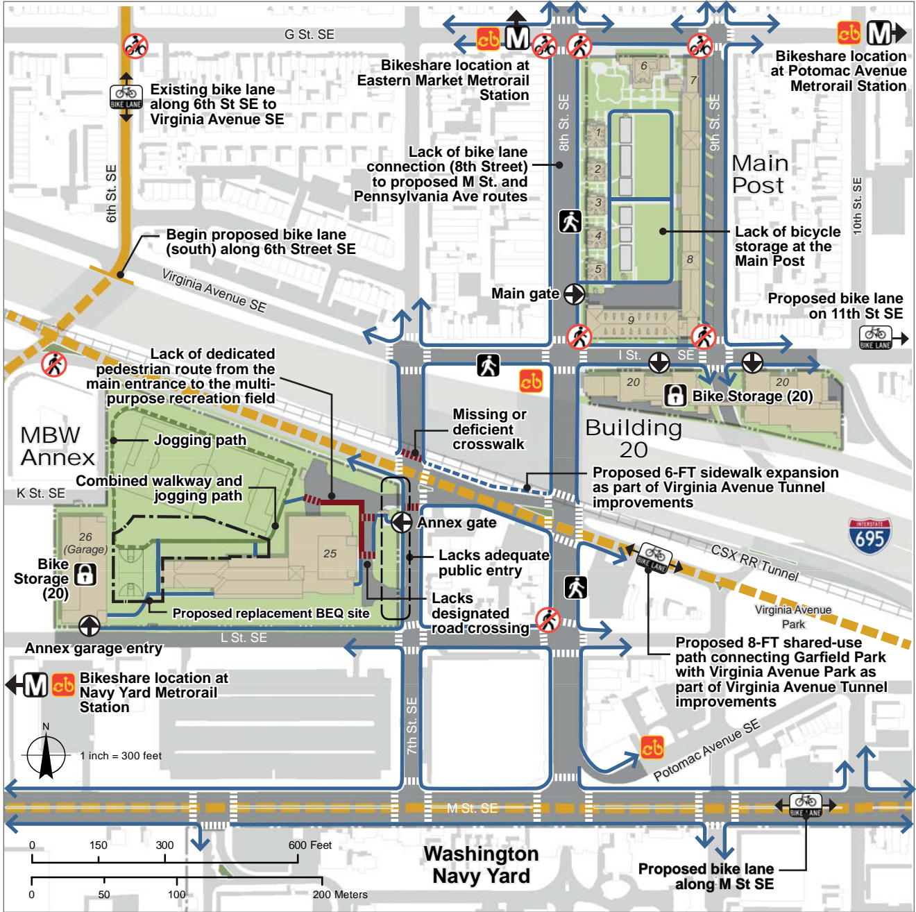
Figure 5-20 Analysis of Pedestrian & Bikeway Facilities
