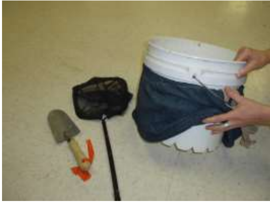
Figure 8.4b Stove-pipe sampler with net and trowel
