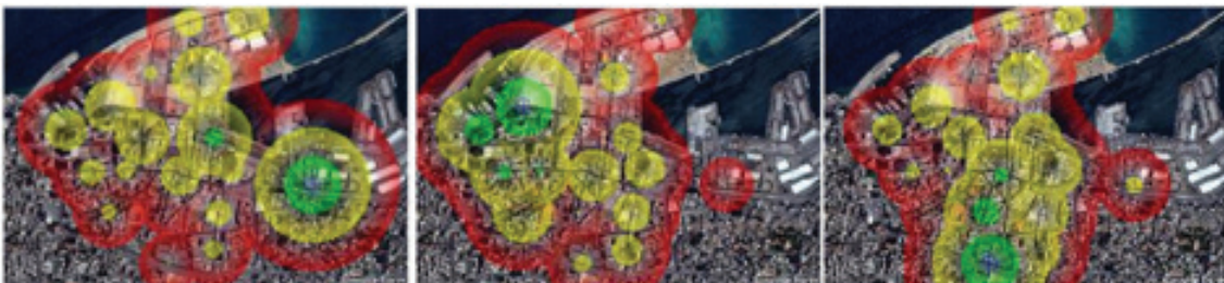
Figure 4: Simulation Results showing time required to reach areas from main station (green 3 min, yellow 6 min, red 9min)
