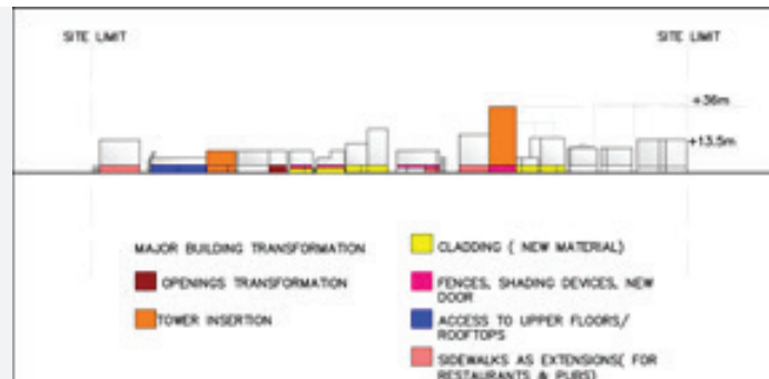
Figure 8: The micro transformation of east elevation of the study area
