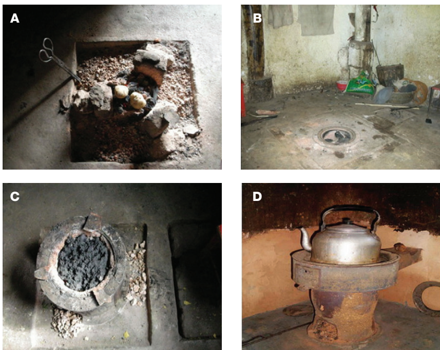
A, B, C, without chimney and the vented stoves popularly used now. D, with chimney.
